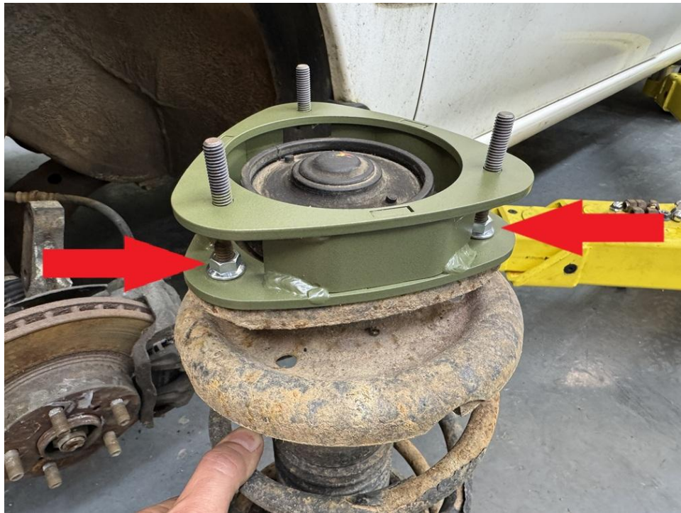
Step 9. Slide strut back into place and loosely install the original 12mm nuts saved from disassembly. (see photo)
