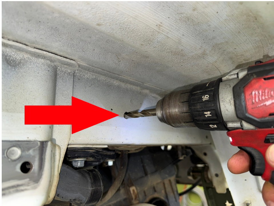
Step 8. We used a compact drill for the rear hole, but a 90* drill would be ideal.
