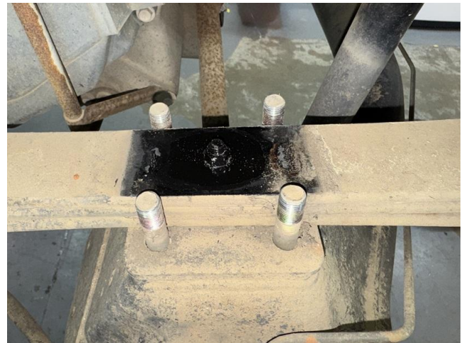
Step 6. Remove bolts holding leaf spring to axle on both driver and passenger side.
