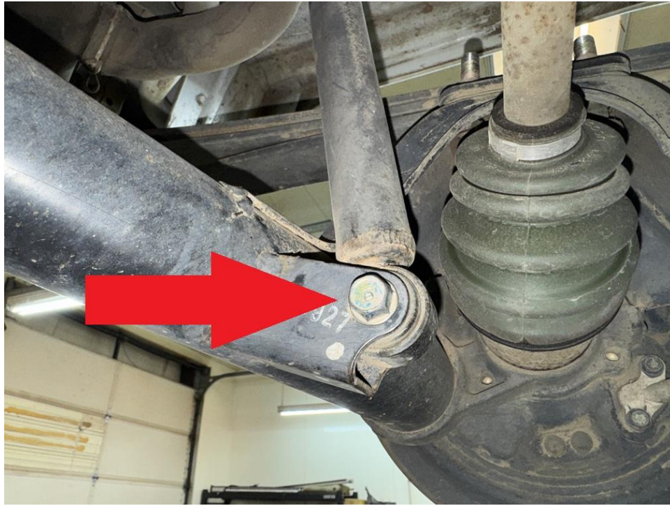
Step 8. Using a pry bar, pop passenger side axle out of transmission.
