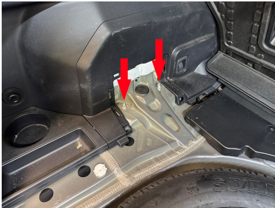
Step 19. Attach spacer to strut using OEM hardware.
