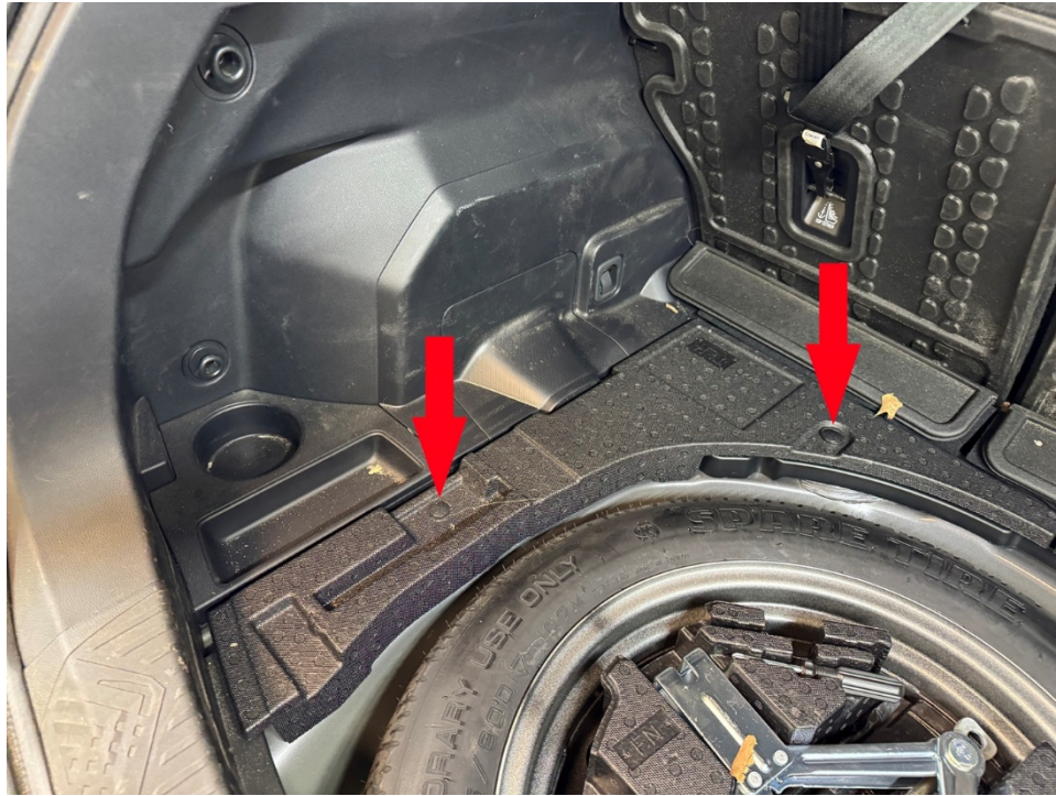
Step 18. Remove 2 nuts holding rear strut to vehicle. Remove strut. (Save hardware)
