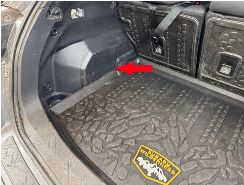
Step 17. Remove plastic clips holding foam piece to trunk floor. Remove foam to allow rear strut access cover to be removed.
