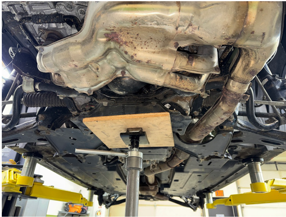
Step 6. Locate and remove bolts and nuts holding the front lower control arm mounts and support brackets. (see photo)
