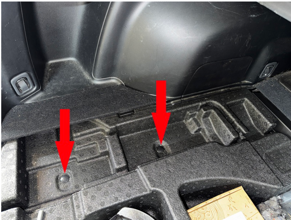
Step 18. Remove plastic cover over rear strut mount.
