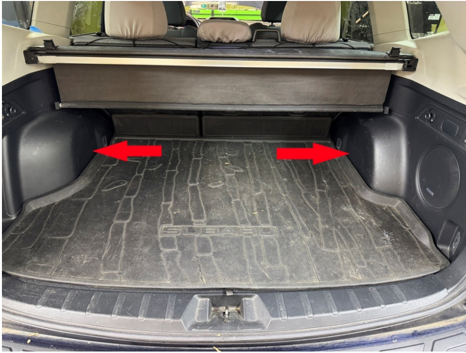
Step 17. Remove plastic clips holding foam piece to trunk floor. Remove foam pieces on both driver and passenger side.
