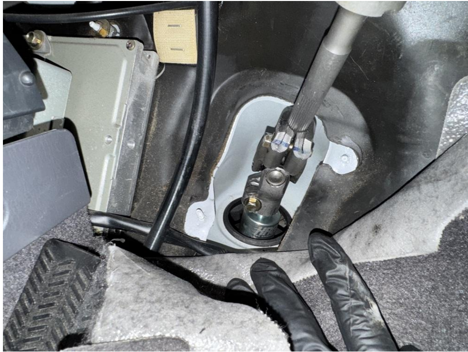
Step 25. Tighten set screws on steering extension.
