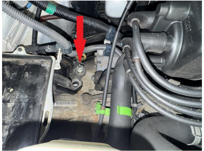
Step 11. Temporarily install M12x80 bolts into transmission. Be sure to allow at least a 1.5 inch gap between the transmission bracket and transmission.
