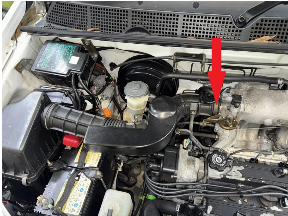
Step 9. Disconnect battery and remove mounting bracket.
