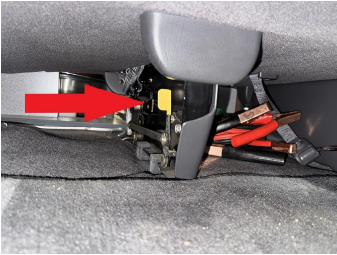
Step 15. Pull carpeting back to reveal driver side rear shock mounting nuts. Remove nuts and have a helper remove the shock from under the car.
