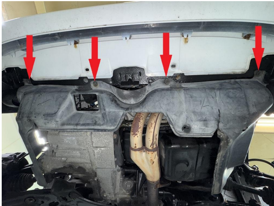
Step 12. Remove plastic clips and screws holding plastic splash guard.
