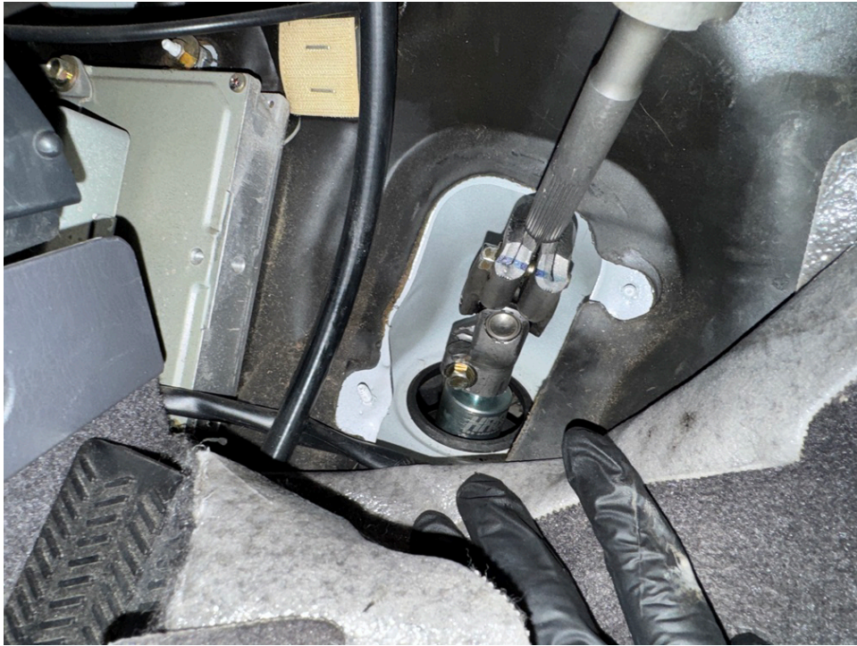
Step 25. Tighten set screws on steering extension.
