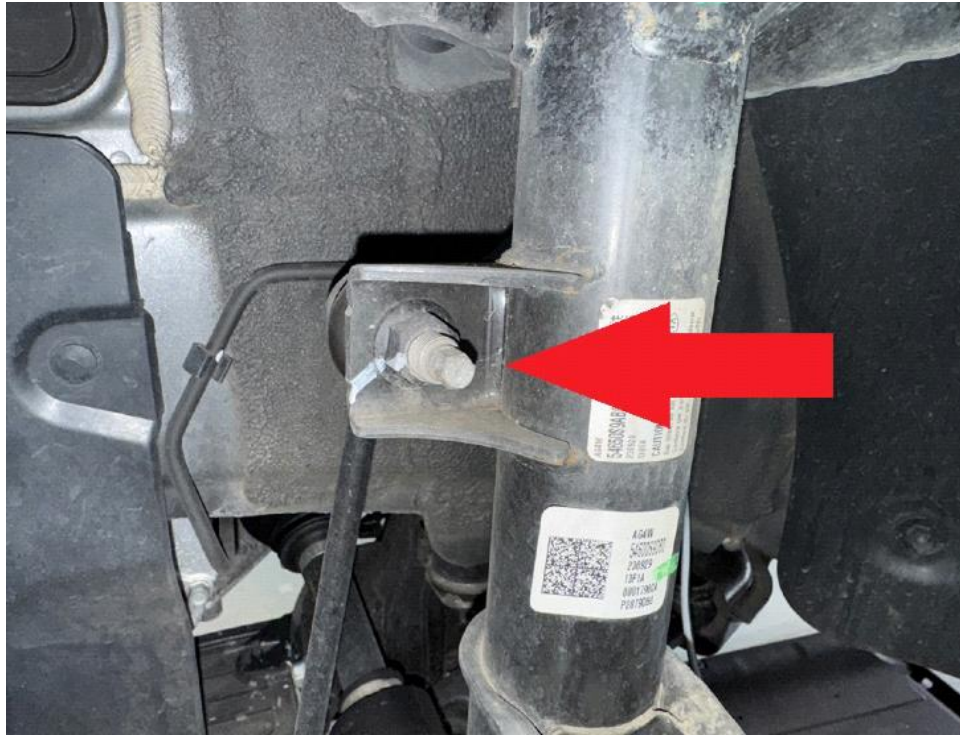
Step 4. Remove brake/ABS lines from driver side strut.
