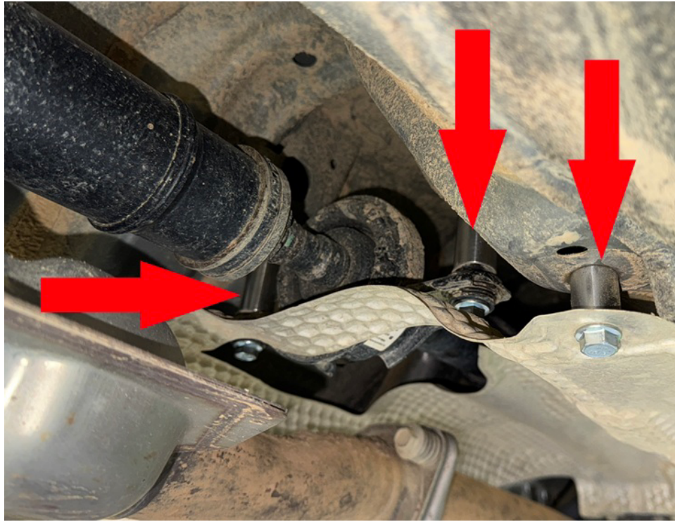
Step 38. Remove bolts holding the brake line, the nut holding the sway bar end link and un-clip ABS wiring from the driver side strut.
