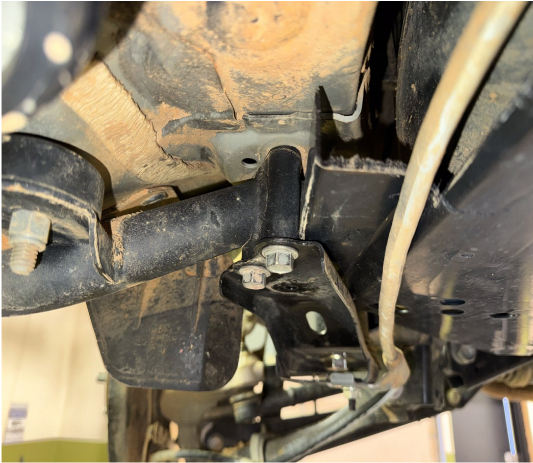
Step 11. Remove bolts holding sway bar link, rear strut, and wheel hub to driver side lower control arm. (see photo)
