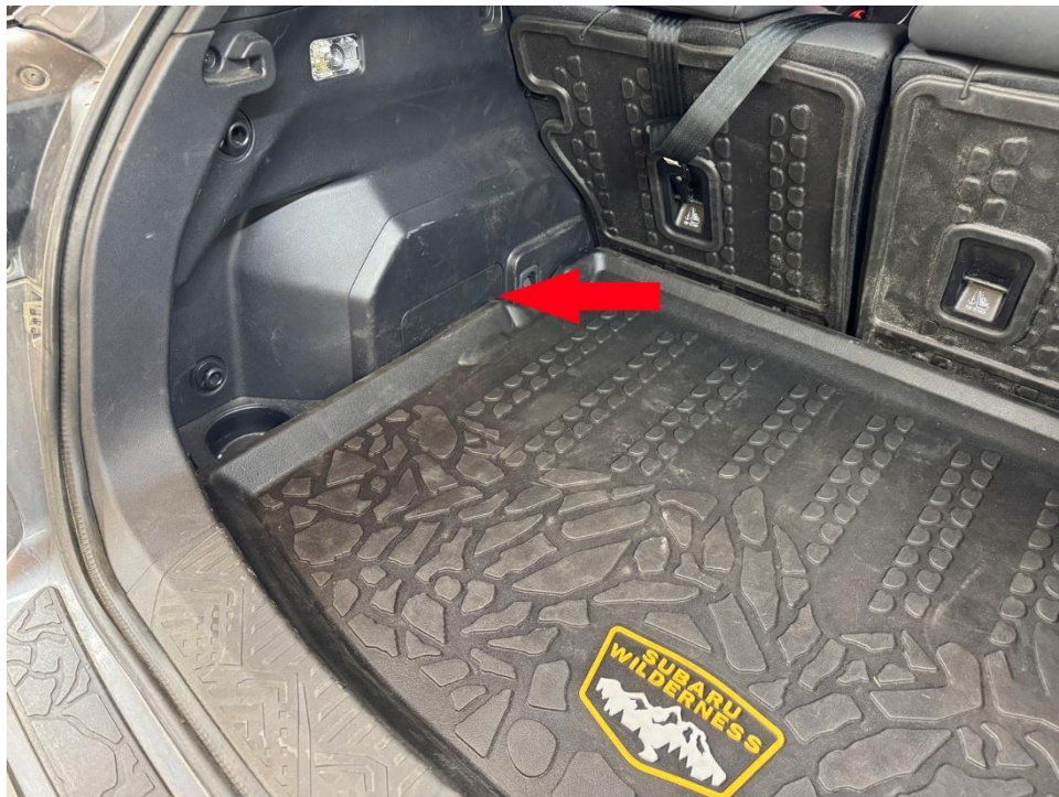
Step 17. Remove plastic clips holding foam piece to trunk floor. Remove foam to allow plastic cover to be removed.
