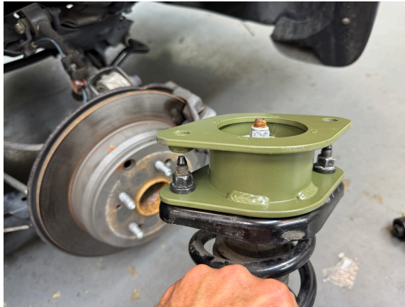
Step 18. Install strut/spacer combo, using bolts included with the kit to secure spacer to rear shock tower.
