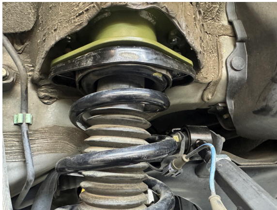
Step 19. Using a large pry bar, move the rear suspension down to align lower strut mounting bolt. Install bolt, torque to 95 ft-lb.
