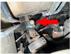
Step 8. Remove 17mm bolts holding engine cradle to frame rails one at a time, temporarily installing M12x120 bolts as you go. Do not tighten bolts at this time.
