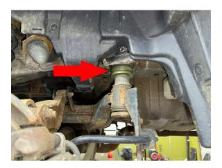
Step 10. Repeat process for remaining 3 subframe bolts/spacers.
