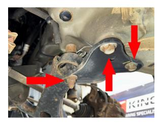
Step 13. Using a 15mm wrench, remove mounting stud as shown. Pry downward on lower control arm to allow stud to be removed.
