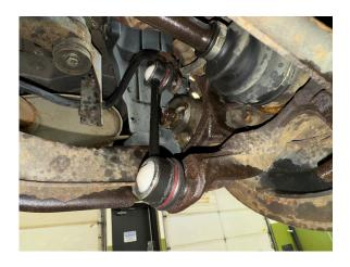
Step 22. Repeat lift spacer and sway bar link installation process on passenger side.
