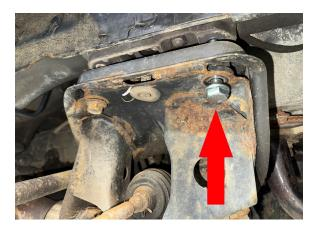
Step 9. Carefully lower engine cradle approximately 1 inch (25mm)
