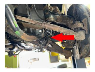
Step 34. Tighten bolts on steering universal coupler.
