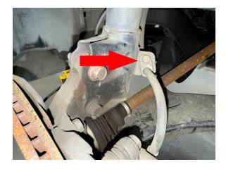
Step 20. Remove nut holding sway bar end link to sway bar. (See photo below)
