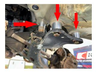
Step 15. Repeat front lower control arm spacer installation process for passenger side.
