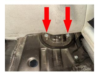
Step 17. Mount the spacer to the strut using the M10 nuts provided in the kit.
