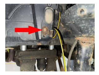
Step 31. Flip ABS mounting bracket upside down and install ABS wire relocation bracket as shown.
