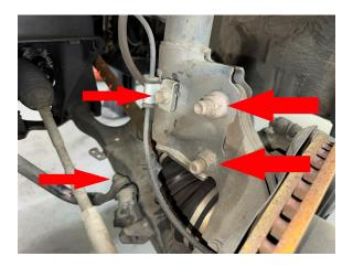
Step 23. Using a heavy hammer, tap strut bolts out.
