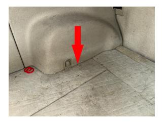
Step 16. Remove 2 14mm nuts holding the rear strut in place. (Save hardware.)
