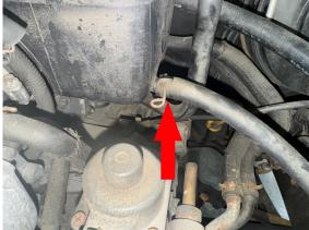
Step 3. Loosen (DO NOT REMOVE) bolt on engine "dog bone" mount as shown:
