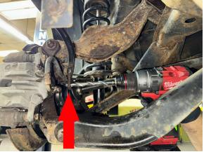
Step 21. Install new sway bar link. Torque nuts to 35 ft-lb
