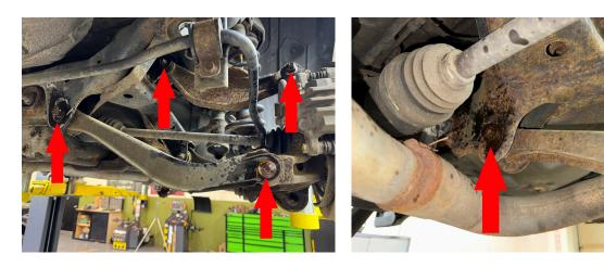
Step 13. Remove both driver and passenger rear sway bar end links. These will not be reused.
