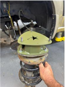
Step 27. Lift strut back into place and bolt in using original hardware. L spacer installs on DRIVER SIDE as shown. Torque nuts to 25 ft-lb.
