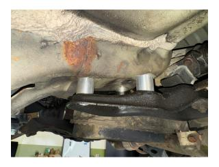
Step 19. Remove 12mm bolt holding brake line from driver side strut.
