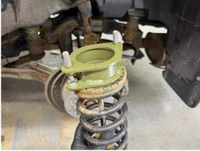
Step 18. Lift strut back into vehicle, lining up the 2 bolts through the strut tower and loosely install the 2 OEM 14mm nuts. (leaving these loose will make aligning the lower mounting bolt easier)
