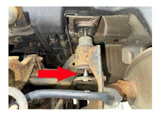
Step 9. Place 2.75x1 M14 spacer between subframe and chassis. Permanently install M14x180 bolt. Torque bolts to 135 ft-lb.
