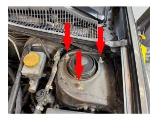
Step 26. Install spacer onto strut using M8 nuts provided in the kit.
