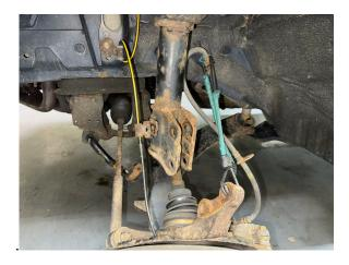
Step 25. Remove 3 12mm from strut top to allow strut to drop out. (Save hardware.)
