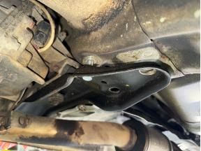
Step 17. Carefully lower transmission support bracket approximately 1 inch (25mm).
