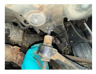
Step 14. Place 3 1.25x1 M14 spacers between front lower control arm mount and chassis as shown. Install M14x150 bolt in place of stud, M14x50 bolts in place of shorter bolts. (see photo)
