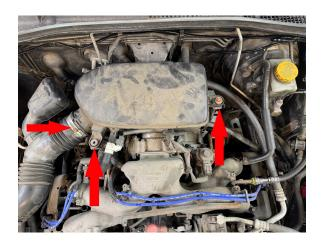
Step 2. Remove emissions hoses from air intake as shown, remove air intake.
