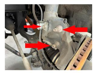
Step 30. Remove bolt holding ABS wire to driver side fender well.
