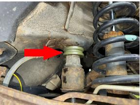
Step 11. Place 1.25x1 M14 Spacers between driver side trailing arm mount and chassis. Install M14x50 bolts. Torque bolts to 90 ft-lb.
