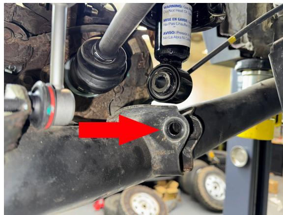
**Warning: these bolts are prone to seizing inside the bushing. If the bolts seize, you will need to cut the bushings and replace them, or replace the strut.**
