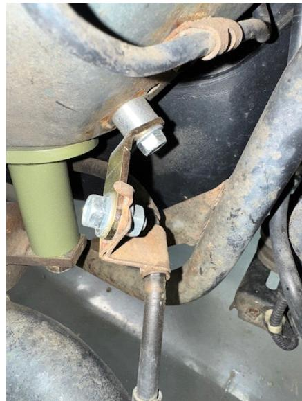
Step 26. Remove 2 M10 bolts in driveshaft carrier bearing.
