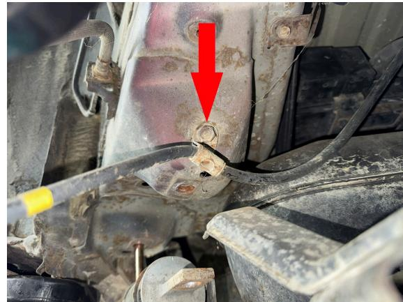
Step 16. Remove 17mm bolts holding trailing arms to body.
