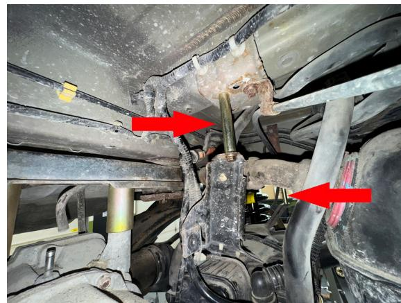
Step 24. Place trailing arm drop bracket between trailing arms and body, install 2 M12x150 bolts. Torque bolts to 85 ft-lb.
