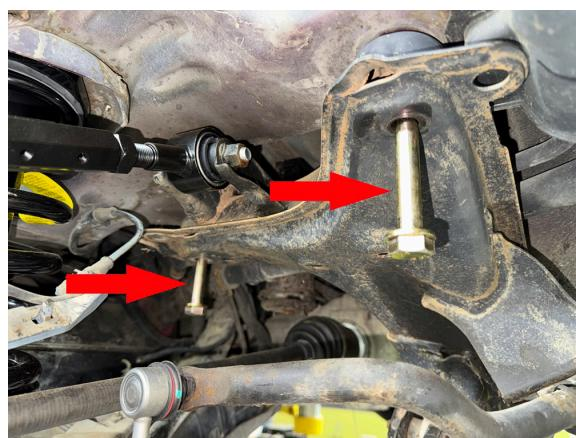
Step 12. Repeat process with remaining 2 rear subframe bolts. (leave 2 bolts in at all times to maintain alignment of
