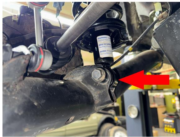
Step 32. Install new adjustable rear upper control arm. Adjust to slightly longer than the OEM arm. Your alignment shop will make final adjustments.
