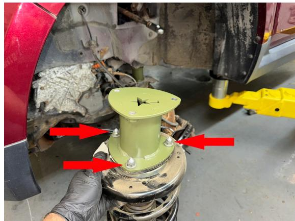
Step 34. Install strut and spacer assembly into shock tower using 3 M10x25 bolts.
