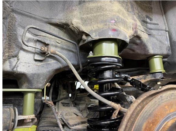
Step 31. Using a pry bar, force lower strut mount into position on lower control arm, install bolt.
