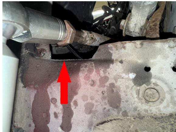
Step 33. Attach spacer marked "L" to top of DRIVER SIDE strut using original hardware.
