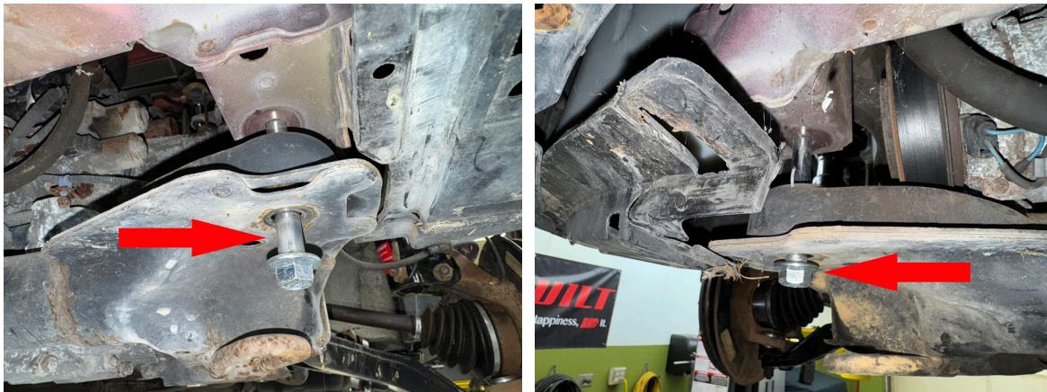
Step 17. Carefully lower engine and subframe assembly down approximately 3 inches.
