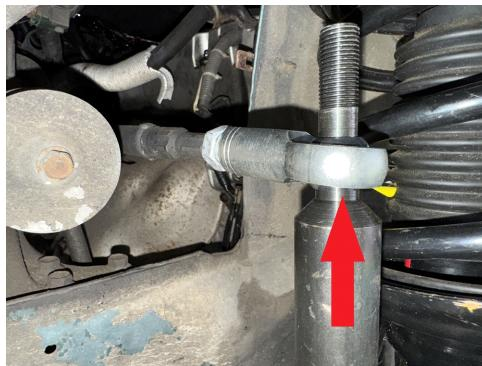
Step 42. Install tapered collar and nut onto tie rod extension as shown in photo: Do not over-torque top nut.
