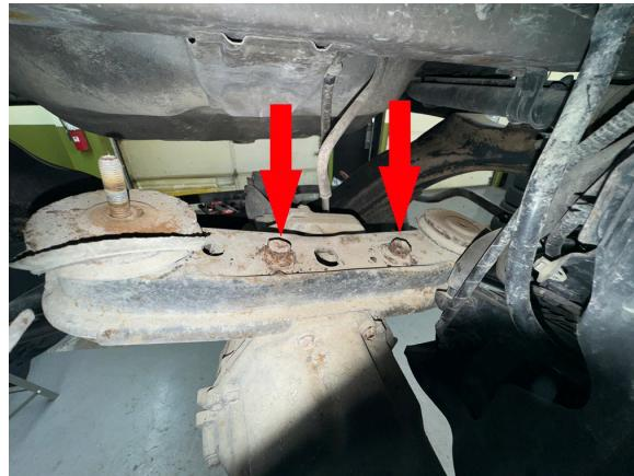
Step 19. Place 2 1.25x3" spacers between differential and differential bracket. Install 2 M12x140 bolts. Torque bolts to 80 ft-lb.
