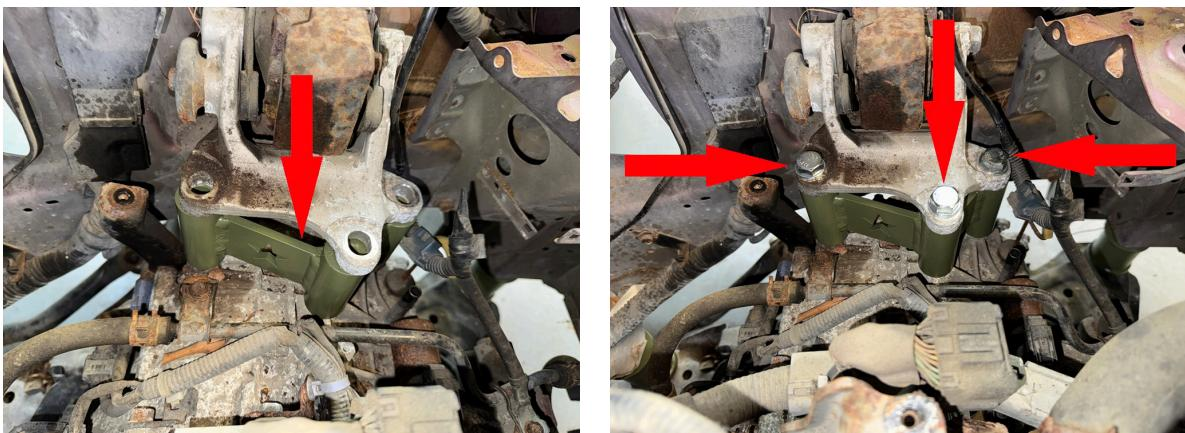
Step 22. Place 0.5x1 and 0.5x1.5 M6 spacers between air box mounting tabs and mounts, secure air box with M6x70 bolts.
