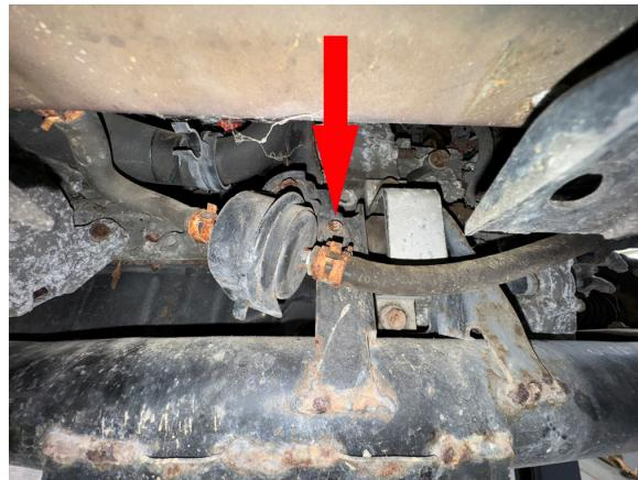
Step 11. Install relocation bracket as shown:
