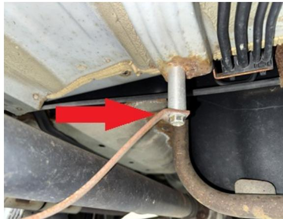
Step 29. Attach rear lift spacer onto driver side strut using original hardware.
