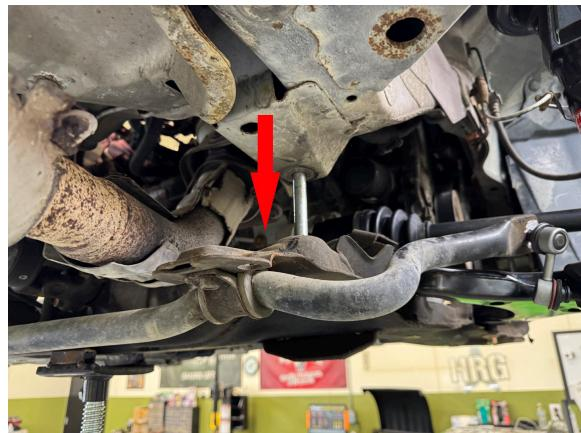
Step 18. Place 2.75x3 M14 spacers between subframe and body one at a time, removing and replacing the bolts as you go.
