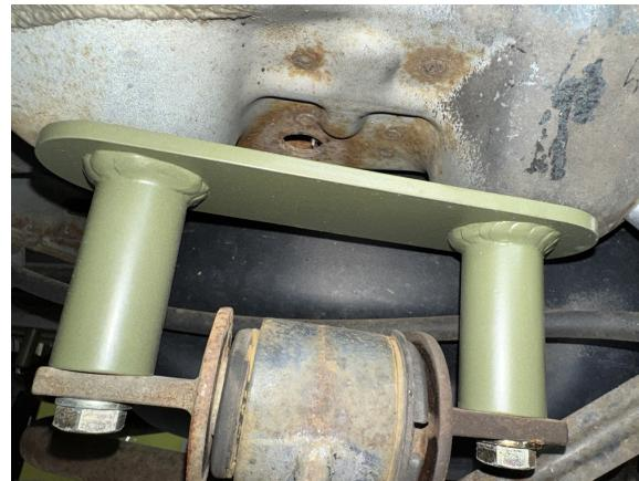
Step 25. Install parking brake cable brackets with M8 bolt (see photo)
