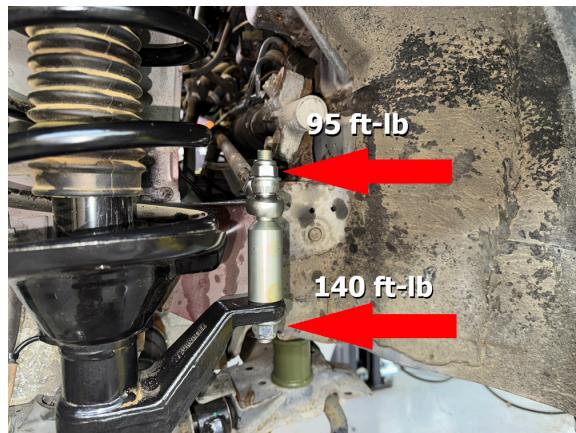
Step 43. Repeat spacer and tie rod end installation for passenger side.
