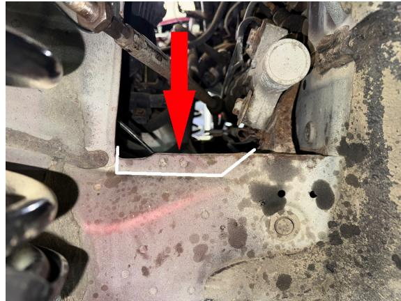
Step 32. Using a body saw or cutoff wheel, cut notch in pinch weld as shown:
