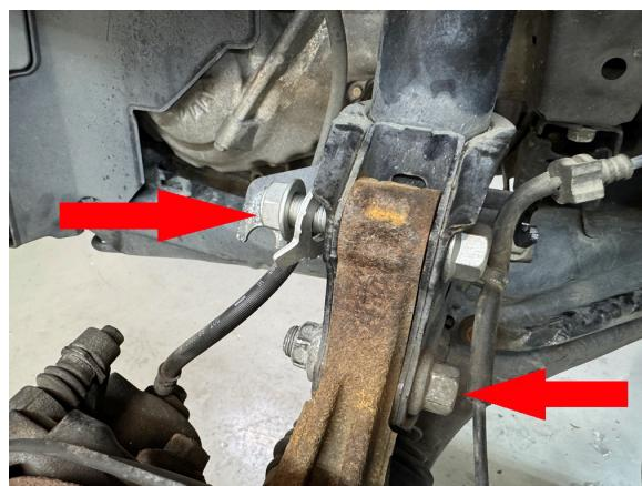
Step 28. Remove cotter pin and castle nut on tie rod end.
