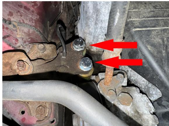
Step 21. Place transmission drop bracket between transmission and transmission mount, install 3 M12x110 bolts. (see photo) (AUTO TRANS SHOWN)
