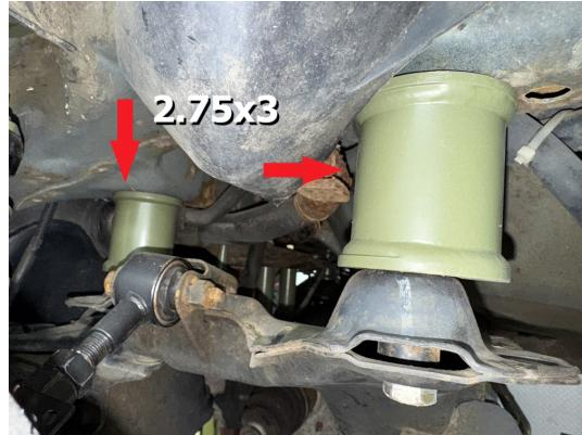
Step 22. Repeat process for remaining 2 subframe bolts. Torque all rear subframe bolts to 95 ft-lb.
