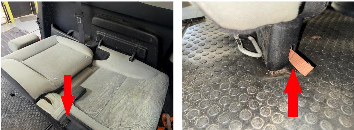
Step 2. Remove plastic panels in rear compartment to allow access to rear strut mounting bolts.
