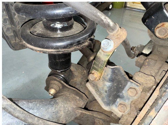
Step 28. Install upper brake line drop bracket (see photo)
