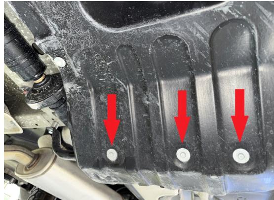
Step 16. Remove 3 M8 bolts holding gas tank bar to body.
