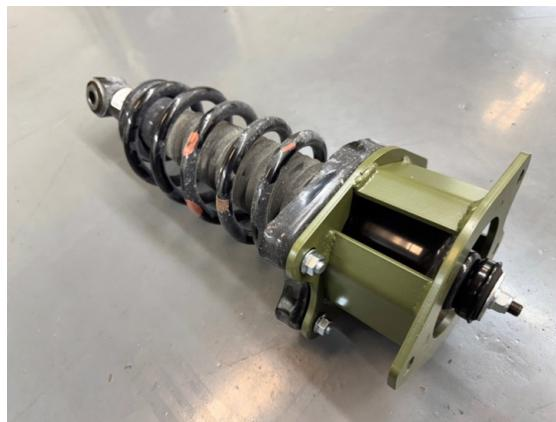
Step 26. Install strut/spacer combination using OEM hardware. Be careful not to cross thread these bolts! Torque OEM bolts to 44 ft-lb. (see photo)
