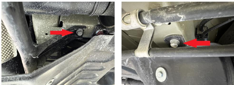
Step 17. Place 3.75x1 M8 spacers between gas tank bar and body, install 3 M8x40 bolts.
