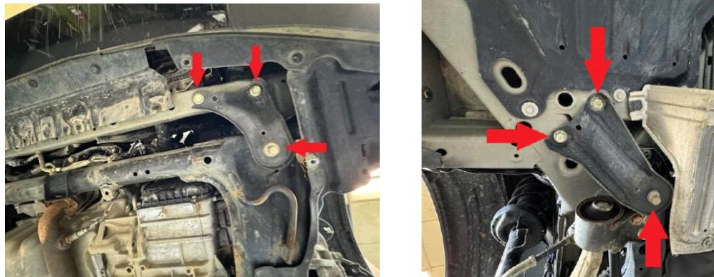
Step 11. Remove the 2 remaining OEM subframe bolts one at a time, lower subframe carefully about 2 inches with floor jack or screw jacks and slip 2.75x2 M14 spacers between subframe and body, installing M14x180 bolts as you go.
