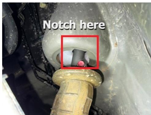
*ALTERNATE METHOD: Using a screwdriver or round bar, bend sheet metal back about 1/4 inch around*
