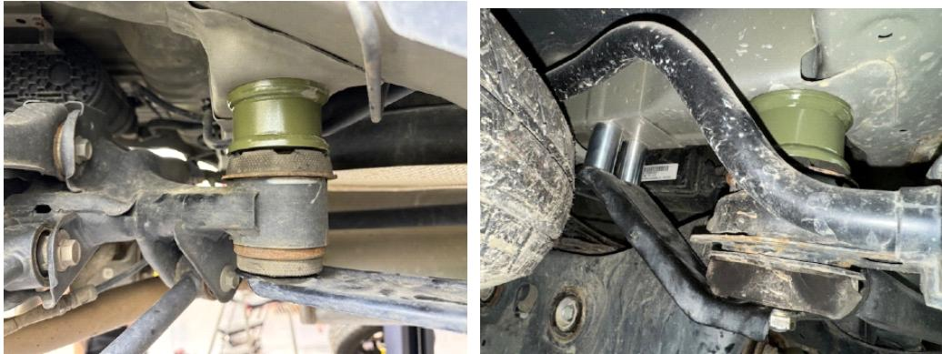
Step 8. Place 1.25x2 M12 spacers between subframe stiffener brackets and body, install 8 M12x70 bolts.
