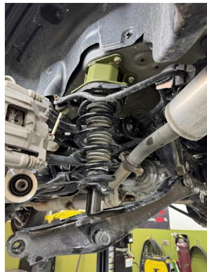
Step 27. Using a floor jack, lift lower control arm until bolt holes line up.
