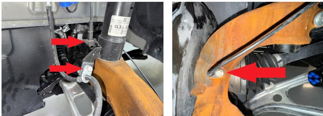
Step 21. Remove nut holding tie rod end to hub, strike knuckle with heavy hammer to dislodge tie rod end.
