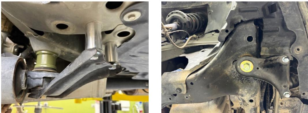
Step 13. Trim fender liner as necessary to fit with lowered subframe, relocate flap to top side of subframe and secure using original hardware. (see photo)
