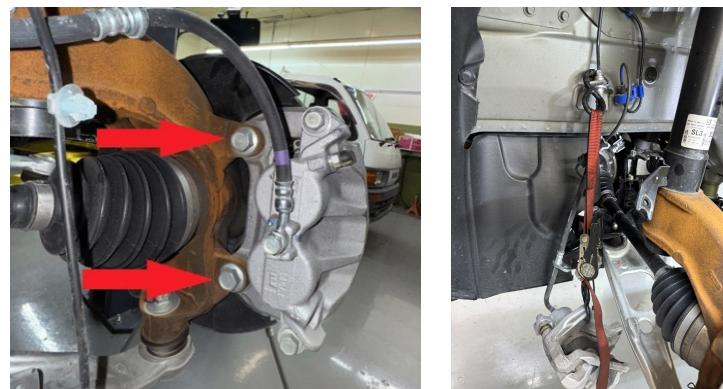
Step 23. Remove brake rotor and axle nut.
