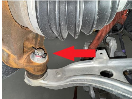
Step 26. Have a helper pry downward on the lower control arm while striking the hub with a large hammer, to separate the ball joint from the hub. This can take dozens of hits. Be careful not to hit the ball joint boot.
