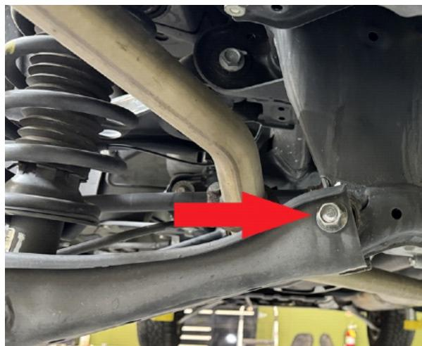
Step 24. Remove 3 bolts holding strut to body and remove strut.
