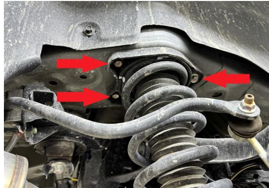
Step 25. Place spacer on top of strut and attach using hardware provided in the kit.
