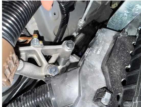
Step 20. Remove brake line and unclip ABS wiring from strut.
