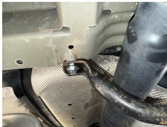
Step 18. Remove rubber rear tailpipe hangers from tailpipe.
