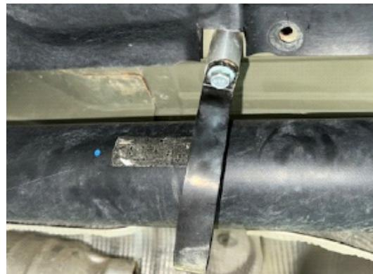
Step 13. Remove 2 M10 bolts holding driveshaft carrier bearing.
