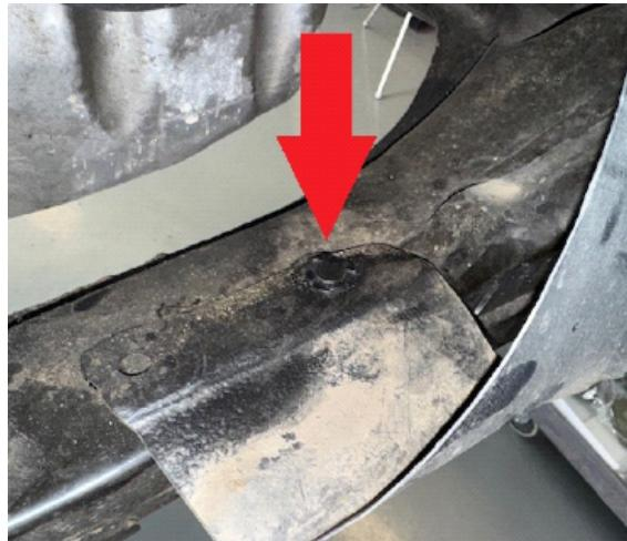
Step 14. Re-install aluminum heat shield, drill new holes and bend as necessary to fit with lowered subframe. Re-attach using OEM hardware.
