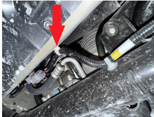
Step 9. Remove the 8 M12 bolts holding subframe stiffener brackets to body. (see photo below)
