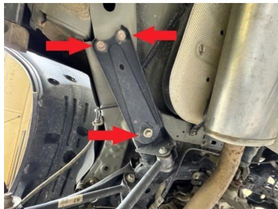
Step 4. Loosen 4 main M14 bolts holding subframe to body, removing only the front 2. Temporarily install 2 M14x180 bolts. This keeps the subframe square and in line when lowering.
