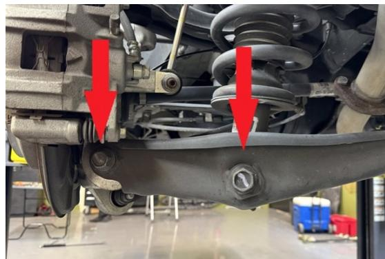
Step 23. Loosen but do not remove bolt holding lower control arm to subframe. (innermost bolt) to allow arm to move freely.
