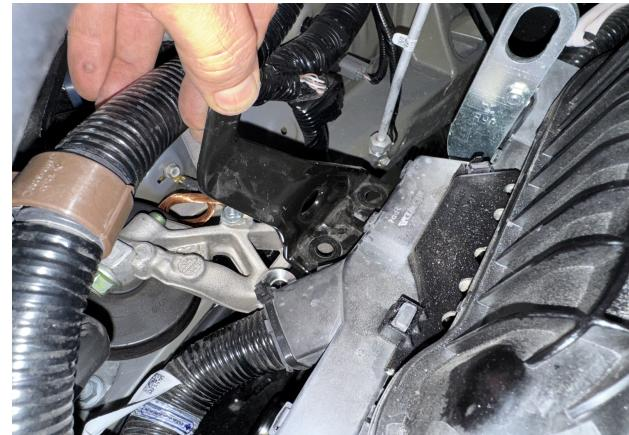
Step 3. Remove air box bolt as shown:
