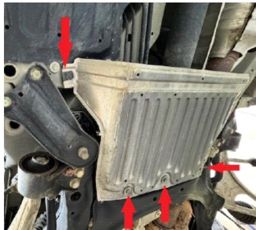
Step 6. Remove plastic clips and 10mm bolts holding aluminum heat shield behind subframe. Save hardware.
