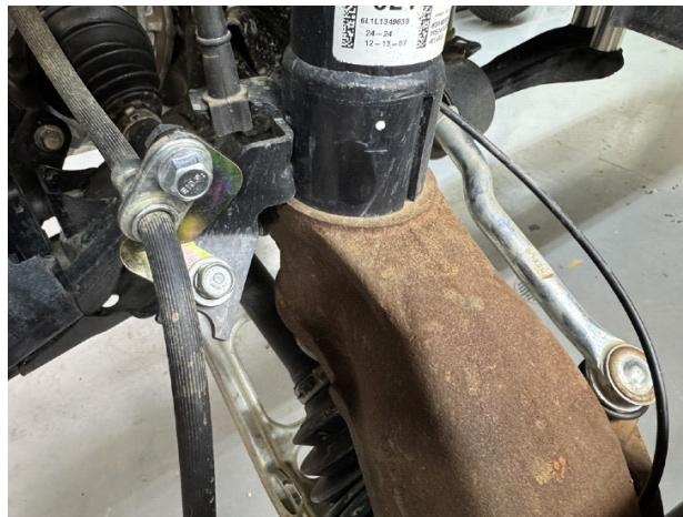
Step 36. Repeat installation process for passenger side. (**sway bar end links will not bolt up until both sides are lifted**)
