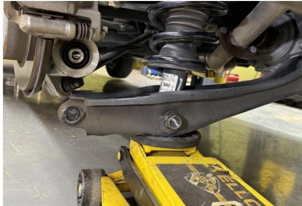
Step 28. Reinstall bolt holding lower control arm to hub. Torque bolts to 135 ft-lb.
