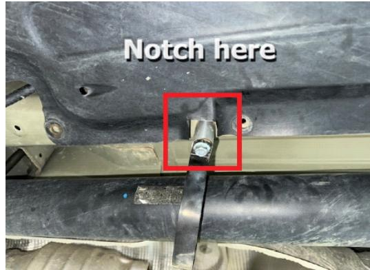
Step 12. Remove bolts holding driveshaft protector, place 0.75x1 M8 spacers between protector and body. (see photo)
