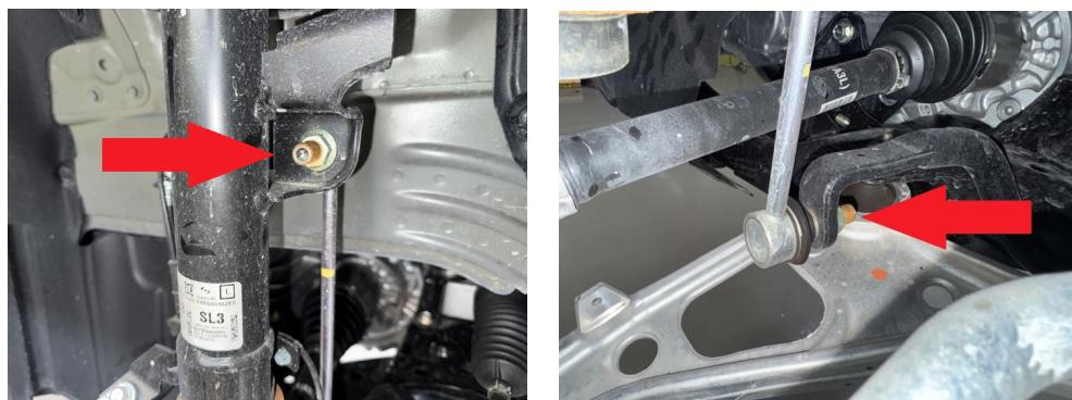
Step 25. Remove lower ball joint nut and cotter pin.
