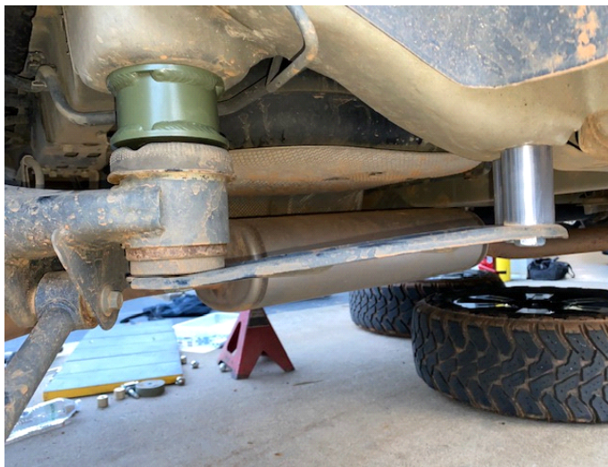
Step 8. Remove bolts holding driveshaft protector, place 0.75x1 M8 spacers between protector and body. (see photo)
