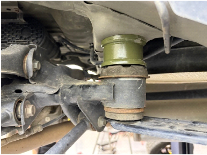
Step 7. Install 8 1.25x2 M12 spacers between support brackets and body, install 8 M12x70 bolts.
