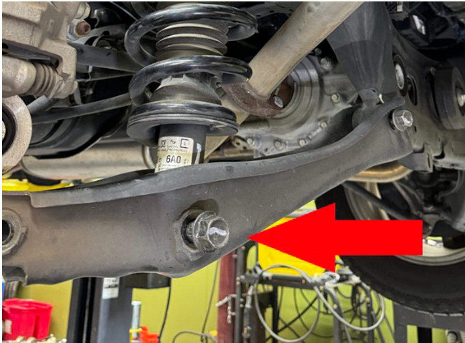
Step 25. Using a floor jack, lift the lower control arm until bolt holes line up.
