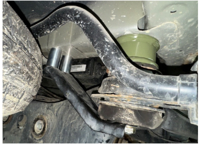
Step 7. Install 8 1.25x2 M12 spacers between support brackets and body, install 8 M12x70 bolts.
