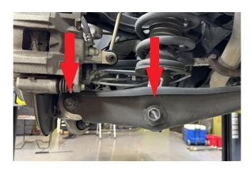
Step 20. Loosen but do not remove bolt holding lower control arm to subframe. (innermost bolt) to allow arm to move freely.
