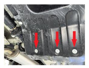
Step 13. Remove 3 12mm bolts holding gas tank bar to body.
