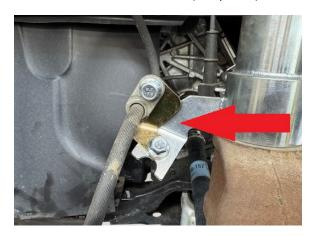
Step 35. Reinstall wheel sensor.
