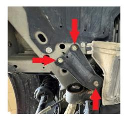
Step 10. Remove the 2 remaining OEM subframe bolts one at a time, lower subframe carefully about 2 inches with floor jack or screw jacks and slip 2.75x2 M14 spacers between subframe and body, installing M14x180 bolts as you go. (This keeps the subframe square and aligned during installation.)
