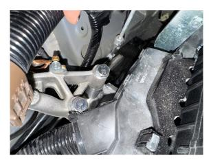
Step 19. Remove brake line and unclip ABS wiring from strut, remove wheel sensor.
