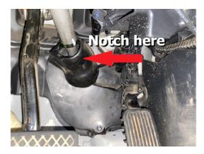
Step 17. Re-install dust cover on steering column below interior dashboard. Double check full rotation of steering wheel to check for any noises or rubbing. Trim as necessary.
