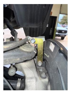
Step 28. Using a crescent wrench, reposition the rear brake line upper bracket in a way that provides additional slack on the brake line.
