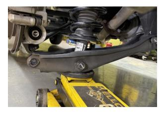
Step 26. Reinstall bolt holding lower control arm to hub. Torque bolts to 135 ft-lb.
