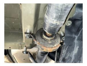
Step 12. Remove 10mm bolts holding plastic under tray to gas tank bar (save hardware).
