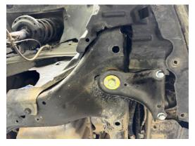
Step 12. Trim and relocate plastic splash shield as necessary to fit with lowered subframe, reinstall clips on top of subframe as shown using original hardware.
