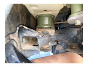
Step 6. Remove the remaining 2 rear subframe bolts one by one, installing remaining 3.5x2" M14 spacers and M14x180 bolts.
