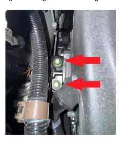
Step 2. Remove bolt on rear outer corner of air box (see photo)
