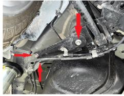
Step 4. Loosen four main M14 bolts holding subframe to body, removing only the front 2. Temporarily install 2 M14x180 bolts in their place. This step will keep the subframe in alignment while being lowered.
