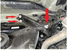
Step 5. Using a floor jack or pole jack, lower the subframe enough to install two of the 4 3.5x2" M14 spacers between subframe and body. Install M14x180 bolts. Be sure to pass bolts through support brackets! (see photos)
