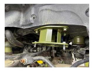
Step 23. Install strut/spacer combination using supplied hardware. Torque bolts to 44 ft-lb. BE CAREFUL NOT TO CROSS THREAD THESE BOLTS!
