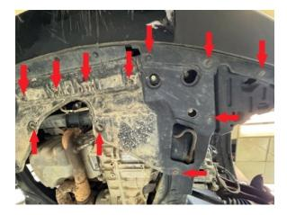
Step 5. Remove plastic clips and 10mm bolts holding aluminum heat shield behind subframe. Save hardware.
