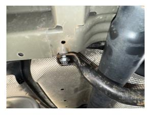
Step 15. Remove rear tailpipe hanger from tailpipes (if applicable).
