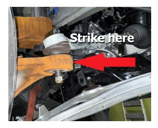
Step 21. Remove lower ball joint nut.
