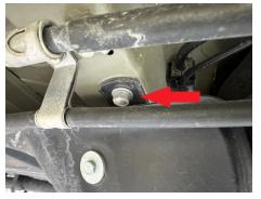
Step 14. Place 3 0.75x1.5 M8 spacers between gas tank bar and body, install 3 M8x60 bolts.
