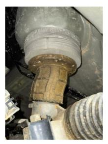
Step 16. Under driver side dash, remove plastic dust cover on steering column. Trim away plastic as necessary to eliminate contact with steering shaft.
