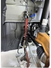
Step 23. Remove brake rotor and axle nut.
