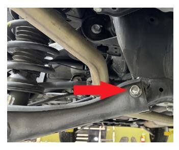
Step 21. Remove three bolts holding strut to body and remove strut.
