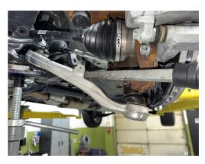
Step 31. Reinstall axle nut, torque to 242 ft-lb.
