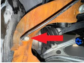
Step 20. Remove nut holding tie rod end to hub, strike knuckle with heavy hammer to dislodge tie rod end.
