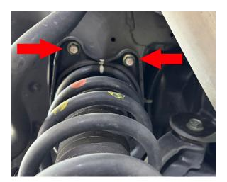
Step 22. Place spacer on top of strut.
