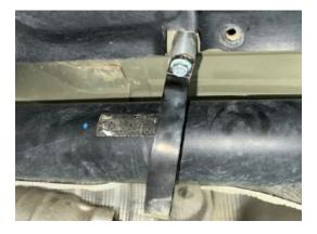
Step 9. Using a plastic cutting tool, notch plastic as shown:
