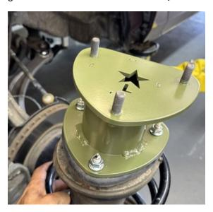
Step 29. Mount spacer, strut, and hub assembly back into shock tower using M10 nuts provided in the kit. Torque nuts to 33 ft-lb.
