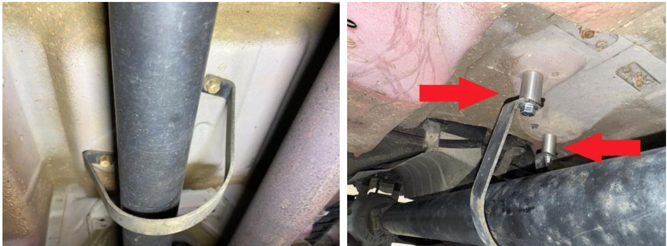
Step 23. Support propeller shaft aka drive shaft with floor jack, carefully remove 2 bolts holding center carrier bearing on propeller shaft, install 2 1x1.5" spacers and 2 M10x60mm bolts.
