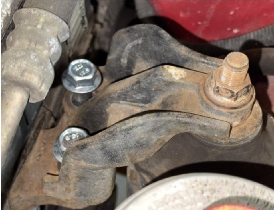
Step 10. Rotate the steering wheel as needed to access bolts holding steering shaft universal joint. Remove 2 10mm bolts in steering shaft universal joint coupler. Save mounting bolts! **Steering coupler will be removed and replaced with a longer one in a later step.**
