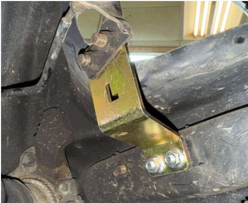
Step 9. Remove 3 14mm bolts holding chassis bar to frame. Remove chassis bar (98-01 only)
