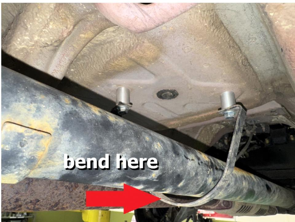
Step 25. Remove rubber exhaust pipe hanger next to carrier bearing and replace with extended hanger provided in the kit.
