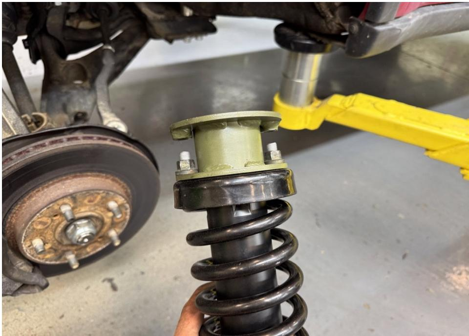
Step 34. Reinstall strut and spacer combo with M10 bolts provided in the kit.
