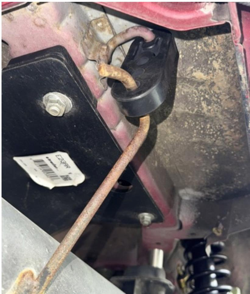
Step 33. Remove bolt holding strut to lower control arm. **Note: these bolts are prone to seizing inside the lower control arm bushing. If the bolts seize, you will need to cut the bushings and replace them, or replace both struts and the rear lower control arms.**
