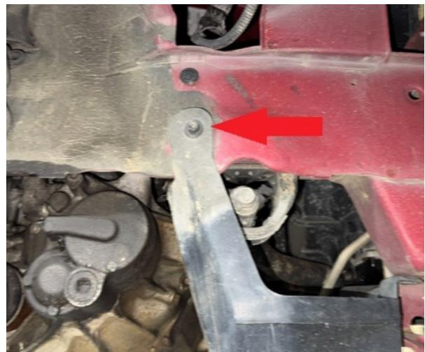
Step 16. Support subframe with floor jack or safety jack. Remove main subframe bolts one at a time and replace them with the bolts included with the kit. There are 4 short bolts and 4 long bolts in the subframe. The short bolts will be replaced by the M14x125, and the long bolts will be replaced by the M12x135
