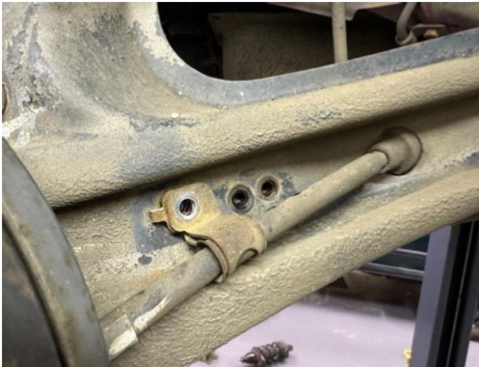
Step 8. Mount brake line relocation bracket as shown using OEM hardware to attach brake hardline to bracket. (see photo) Reinstall bolt holding parking brake cable to trailing arm.
