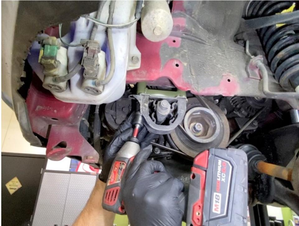
Step 17. Remove steering coupler from steering rack.
