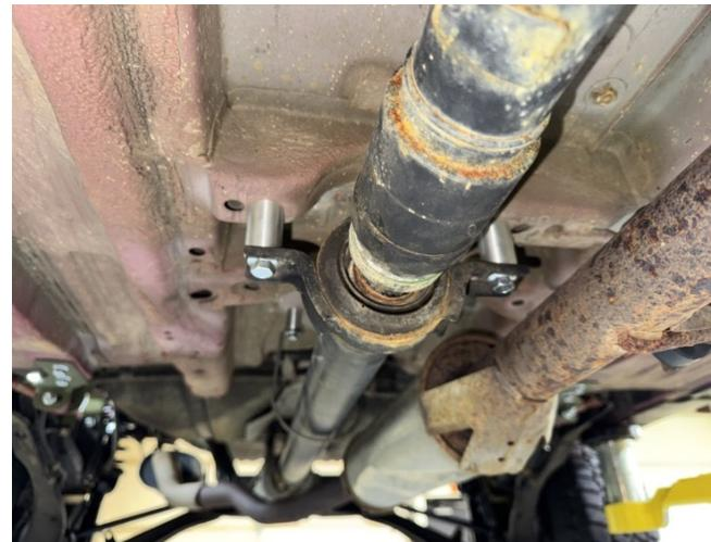
Step 24. Using a pry bar, bend loops to clear driveshaft if necessary.
