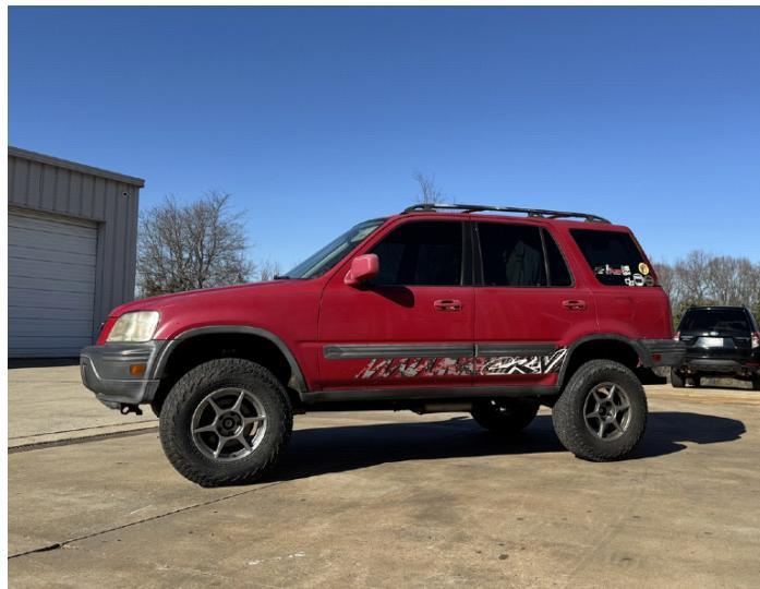
**Installing a lift kit will change the suspension geometry and will require a 4 wheel alignment. Failure to perform a wheel alignment will result in unsafe handling characteristics, accelerated tire wear, and a significant reduction in fuel mileage.**
