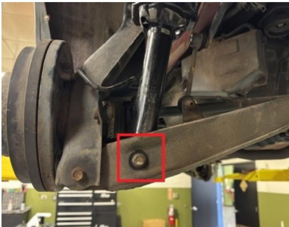
Step 34. Remove nut holding rear sway bar link to lower control arm (if applicable) allowing arm to drop down.
