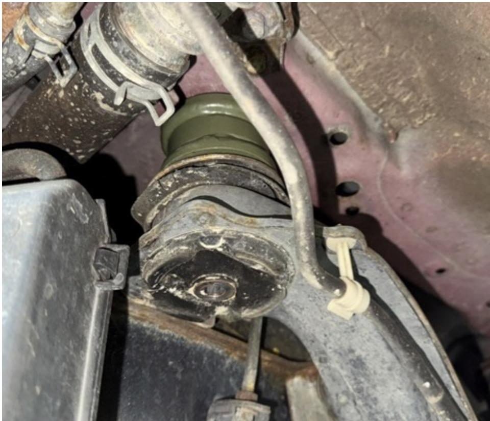
Step 7. Remove the bolt holding parking brake cable and 2 bolts holding brake hardline to trailing arm. (see photo)
