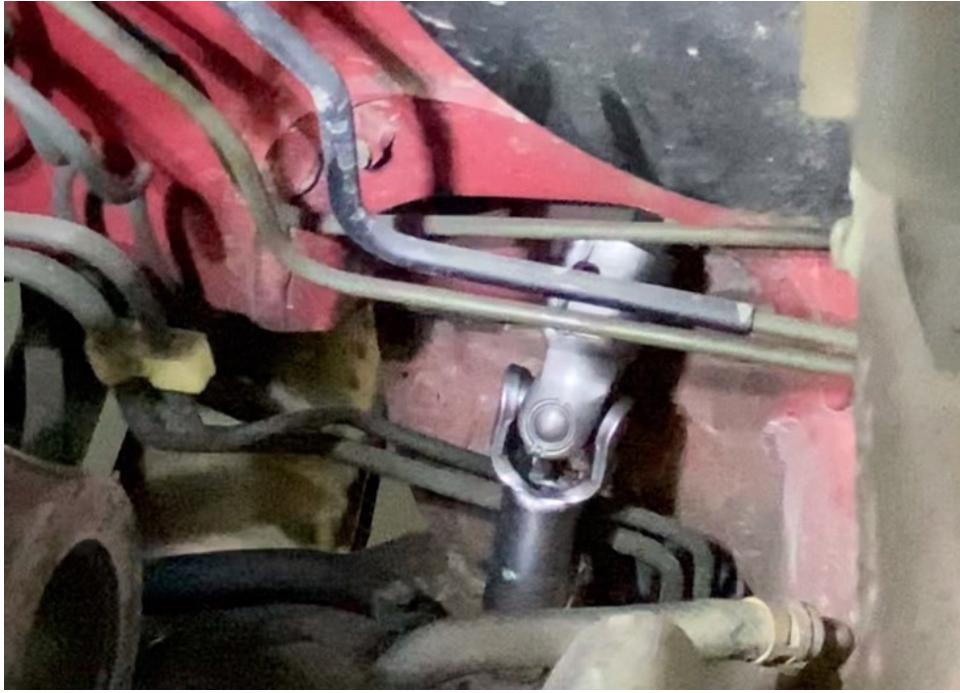
Step 19. Release seat belt holding steering wheel, and rotate wheel as needed to allow access to the coupler bolts. Tighten coupler bolts.
