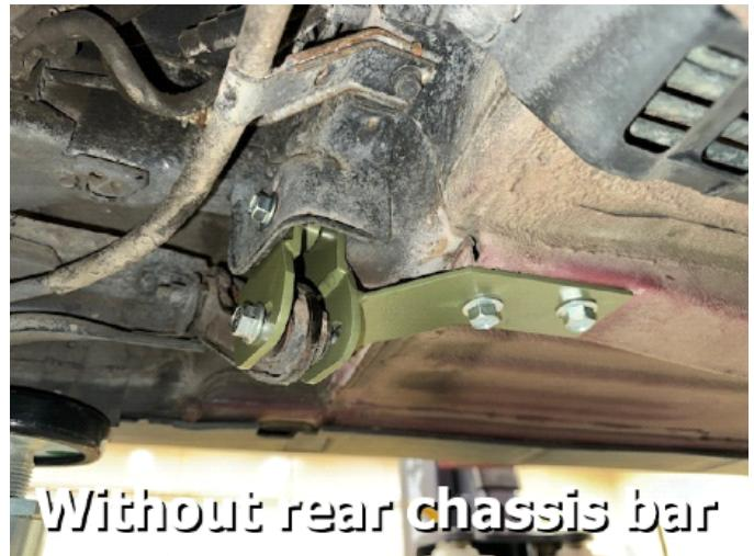
Step 25. Install 3" trailing arm spacers and M12x140mm bolts. (see photo)
