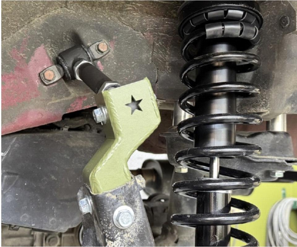
Step 31. Install new adjustable upper control arm in place of original control arm. Take care when installing the 2 14mm bolts holding the upper control arm to the body, as these are prone to cross-threading. Do not mount upper control arm to camber arm relocation bracket at this time.
