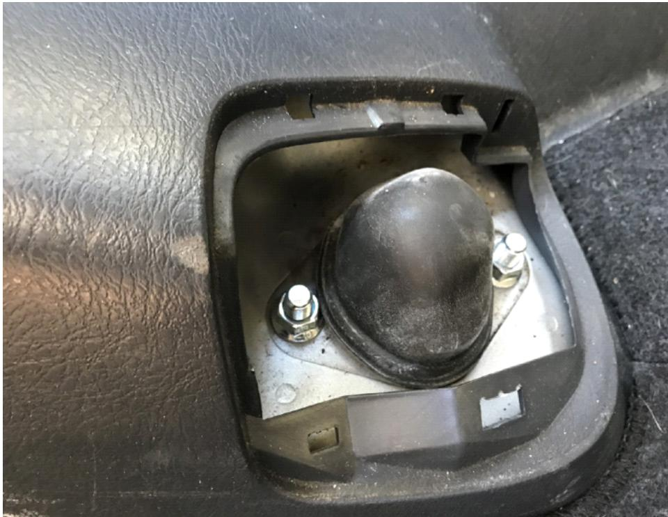
Step 36. Attach 3.5" lift spacer to strut using the OEM Honda nuts.
