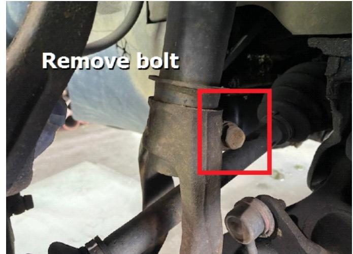
Step 27. Remove nut holding sway bar end link to lower control arm.
