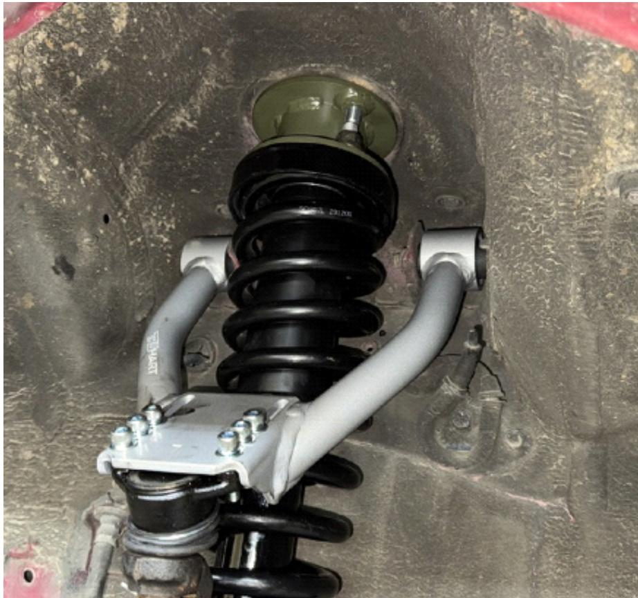
Step 39. Using a floor jack, compress suspension to align upper ball joint and knuckle.
