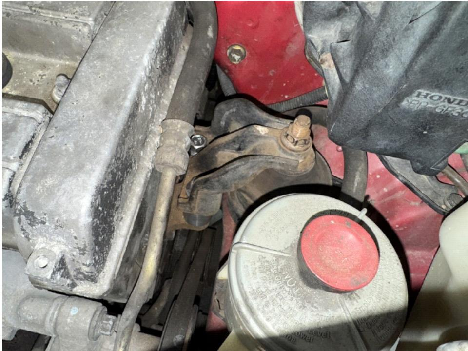
Step 22. Remove 4 12mm bolts holding driveshaft safety loops to body. Install 4 0.75x1" spacers and M8x40 bolts as shown.
