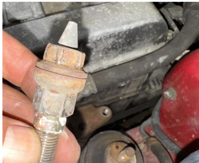
Step 7a. (Manual transmission) Remove transmission mounting bracket and remove studs from transmission case using same technique as removing engine studs. Do not remove transmission mount from frame rail.
