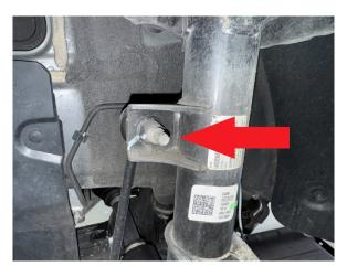
Step 4. Remove brake/ABS lines from driver side strut.
