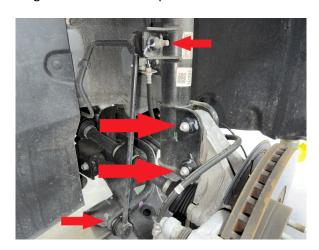
NOTE: Do not allow the hub to fall loose, as the axle may come out of the inner
