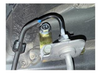
Step 5. Disconnect rear sway bar from lower control arm.
