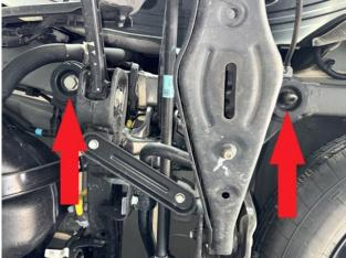
Step 27. Place 2 "G" spacers between subframe and body on FRONT 2 bolts. Tighten bolts.
