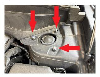
Step 8. Attach lift spacers onto strut using supplied M10 nuts as shown.
