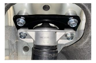
Step 14. Remove 2 bolts holding driver side trailing arm to body.
