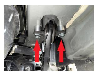
Step 17. Place rubber isolator over rear spring spacer.
