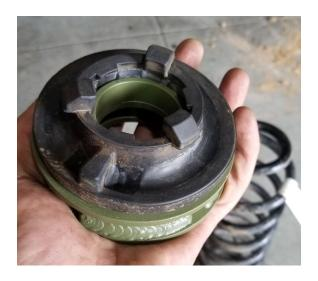
Step 18. Install spring and spacer. Be sure to rotate the spring so that it fits neatly in the relief cut in the lower rubber isolator. (see photos)
