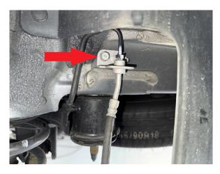
Step 4. Install brake line relocation bracket as shown:
