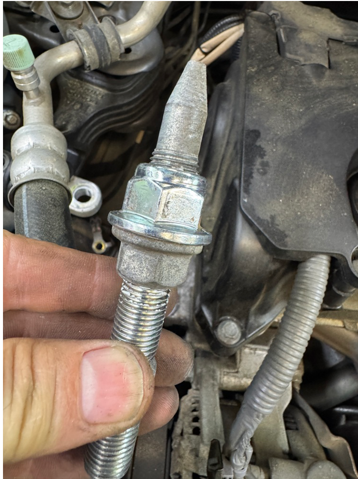
Step 8. Reinstall engine mount. Temporarily install M14x100 bolt to support engine while lowering subframe.
