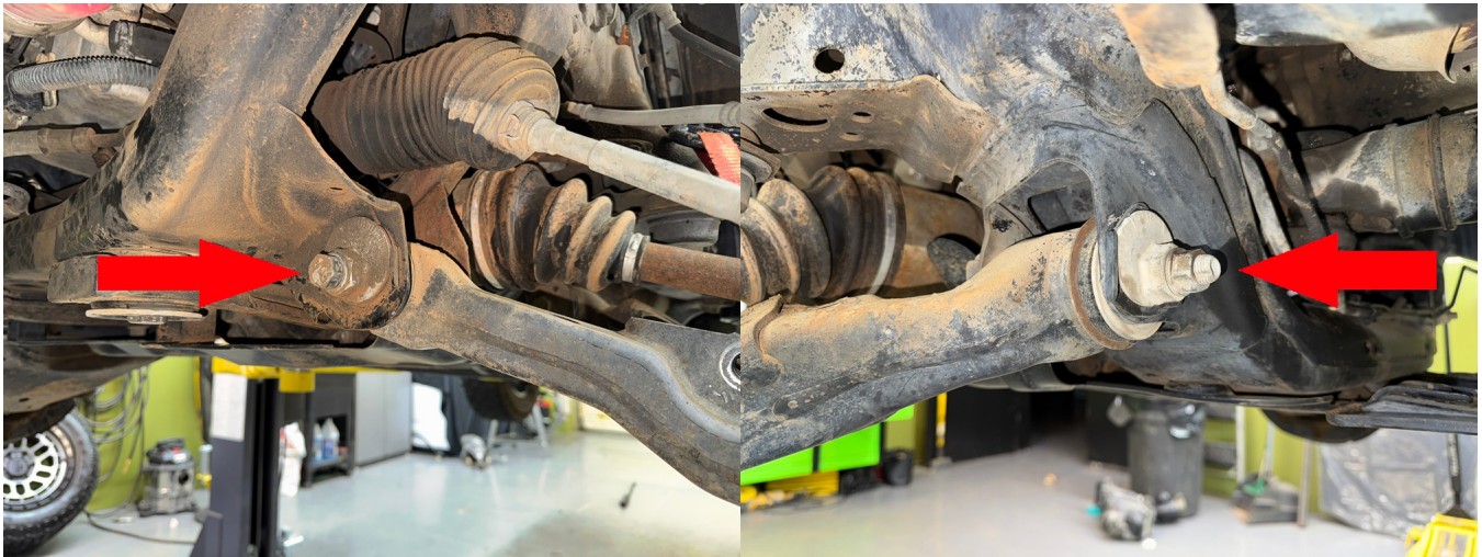
Step 10. Remove sway bar end link nut and loosen upper ball joint nut.
