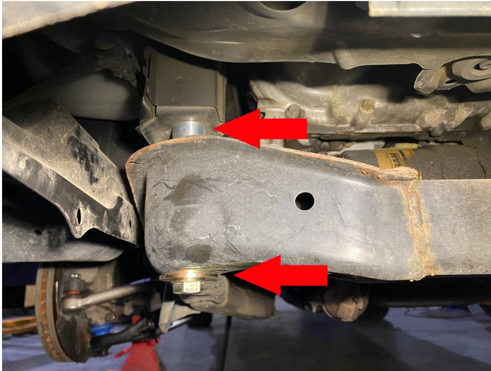
Step 11. Remove 2 bolts and 1 nut on driver side front lower control arm.
