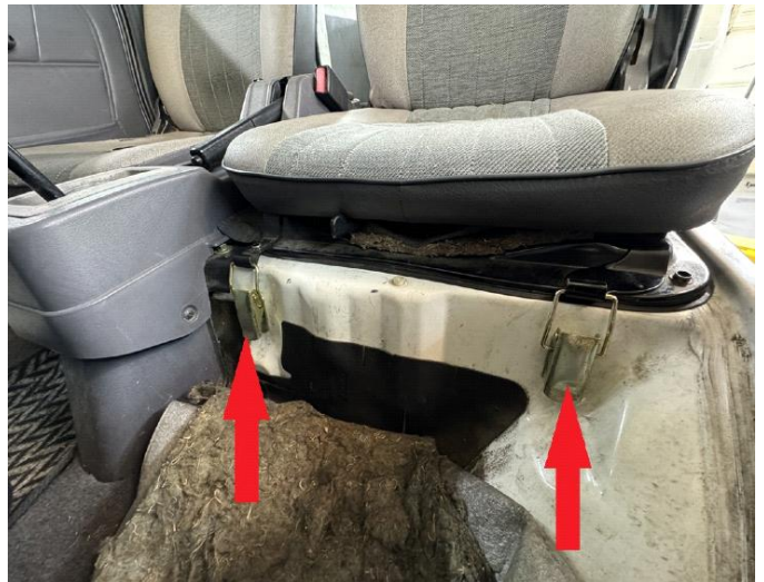
Step 22. Pull back carpet and lift up the bottom of the passenger side seat. Pull forward and up to remove seat bottom.
