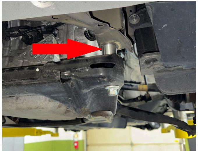
Step 16. Remove bolts holding transmission mounting bracket to frame rail. Remove transmission mount.
