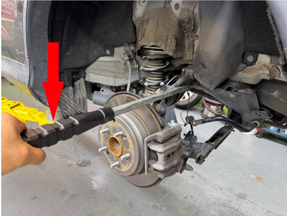
Step 19. Install adjustable rear upper control arms at this time. Adjust arms to be about  $\frac{1}{4}$ " longer than the OEM arms.
