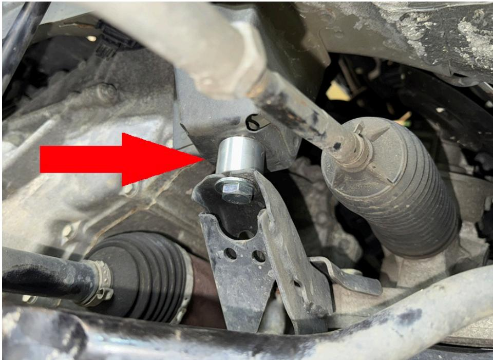
Step 15. Remove all subframe bolts one at a time and place 1.25x1 M14 spacers between subframe and chassis. (see photos) Torque all main subframe bolts to 110 ft-lb.
