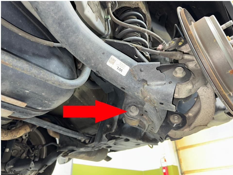
Step 16. Attach spacer to strut using OEM hardware.
