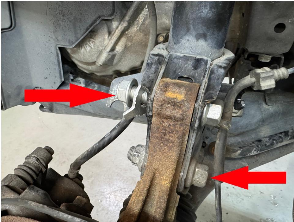
Step 35. Install brake line bracket onto strut as shown:
