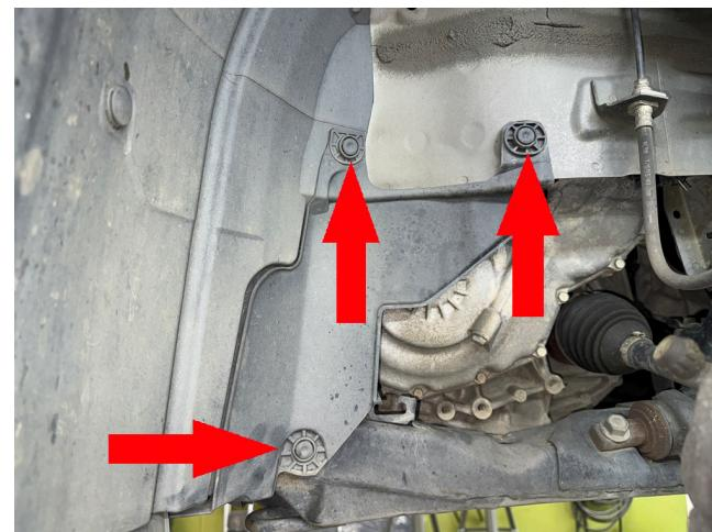
Step 10. Starting with the driver side front, Remove the main subframe bolt and temporarily replace with an M14x150 bolt. Repeat for passenger side front bolt.
