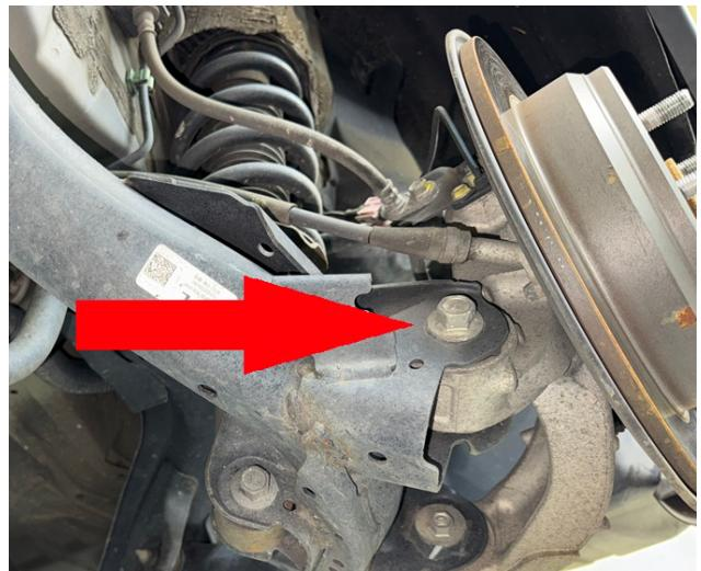
Step 15. Remove driver side rear lower strut bolt, remove rear strut. Repeat on passenger side.
