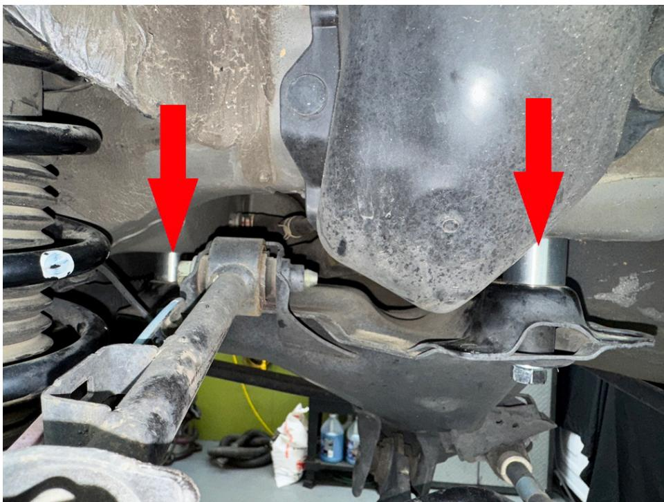
Step 13. Remove M10x140 bolt holding rear differential bracket to chassis and place 2.75x1 M10 spacer between differential bracket and chassis. Permanently install bolt. Torque to 49 ft-lb. Repeat for remaining bolt.
