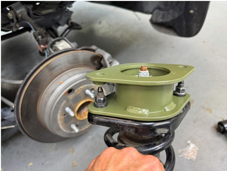
Step 17. Install strut/spacer combo, using bolts included with the kit to secure spacer to rear shock tower.
