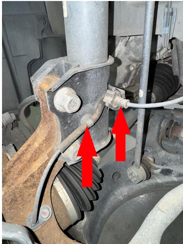
Step 26. Remove bolts connecting strut to knuckle. Save hardware for reinstallation.
