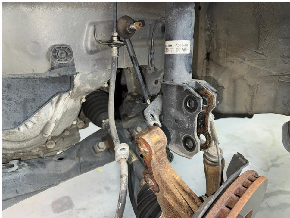
Step 29. Remove plastic panels to gain access to strut mounting bolts.
