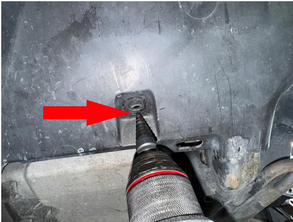
Step 20. Trim plastic splash shield as shown to fit with lowered subframe, reinstall using original hardware.
