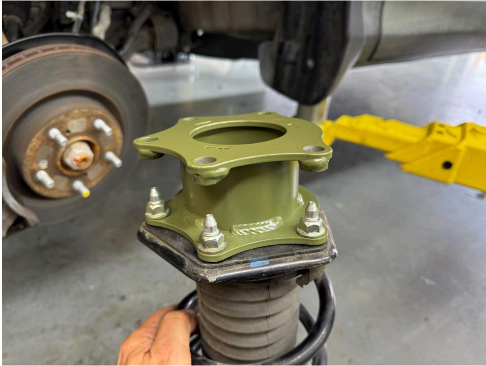
Step 32. Reinstall strut to shock tower using supplied M10x25mm bolts. Torque nuts to 33 ft-lb.
