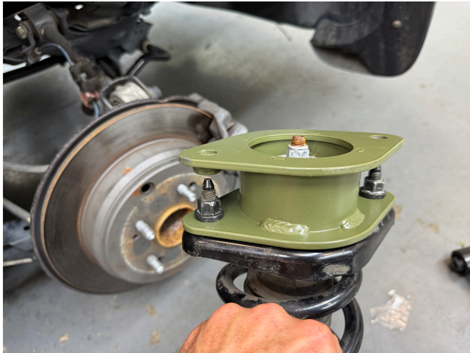
Step 22. Install strut/spacer combo, using bolts included with the kit to secure spacer to rear shock tower.
