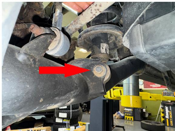
Step 12. Loosen bolts on rear lower control arm to allow suspension to drop.
