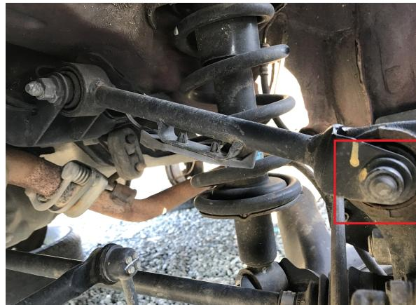
Step 18. Using a floor jack, lift up on rear lower control arm until upper control arm lines up with wheel hub.
