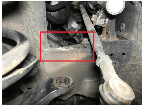
Step 9. Reinstall strut, using M10x25 bolts through the top and into the spacer.
