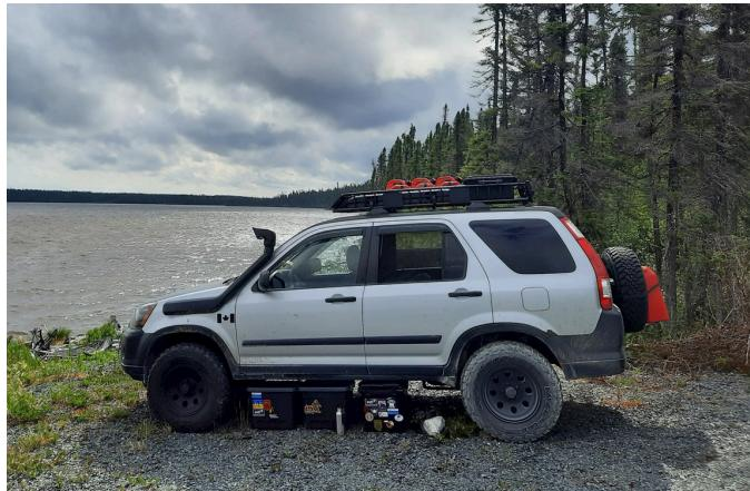
**Note:** Vehicle may appear to sit very high after first installing the lift kit. This is normal and will drop once the vehicle is rolled back and forth. If vehicle still sits extremely high, loosen all suspension arm bolts, roll the vehicle back and forth, and retighten with vehicle on the ground. Due to the wide variety of aftermarket shocks and springs, actual results may vary.
