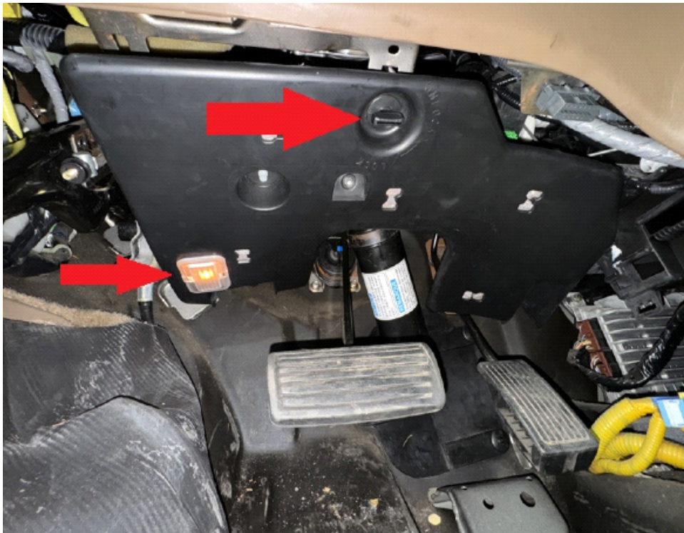
Step 13. Remove plastic cover over steering column.
