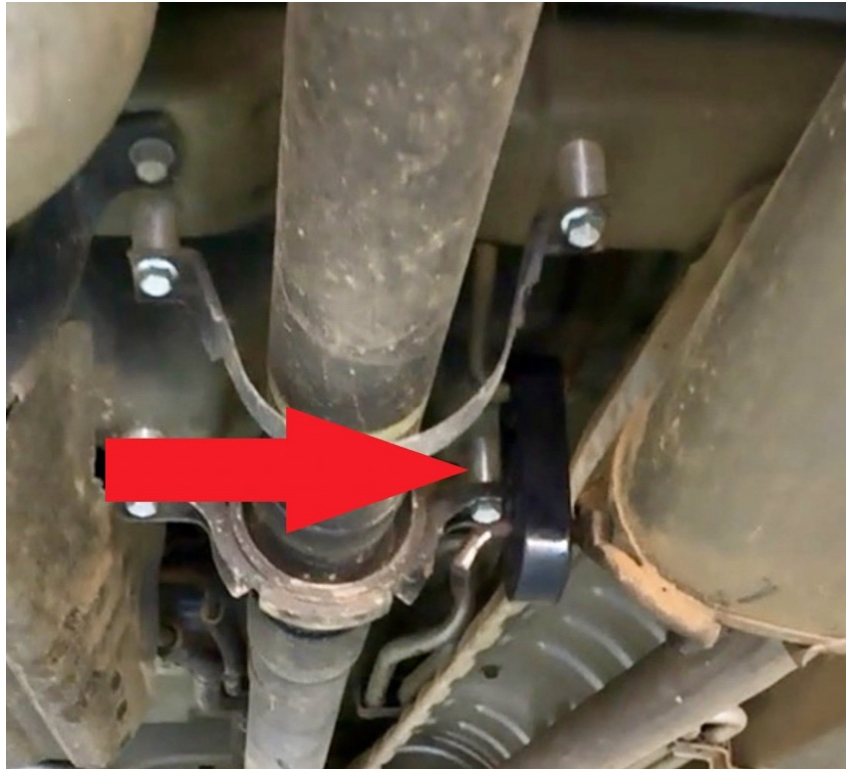
Step 13. Remove upper and lower bolts holding driver side shock absorber.
