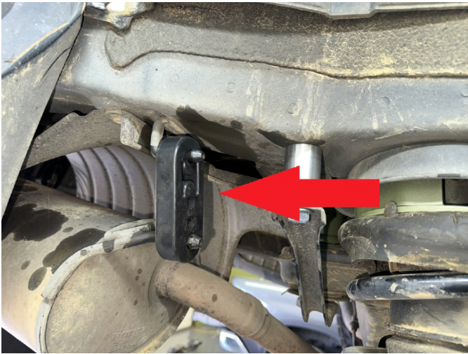
Step 12. Install 1 more exhaust hanger on mid pipe as shown:
