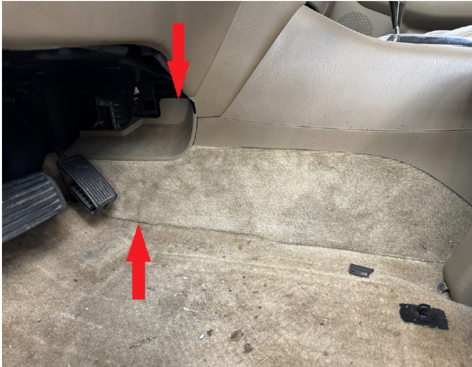
Step 12. Under driver dash, remove plastic cover, disconnect light
