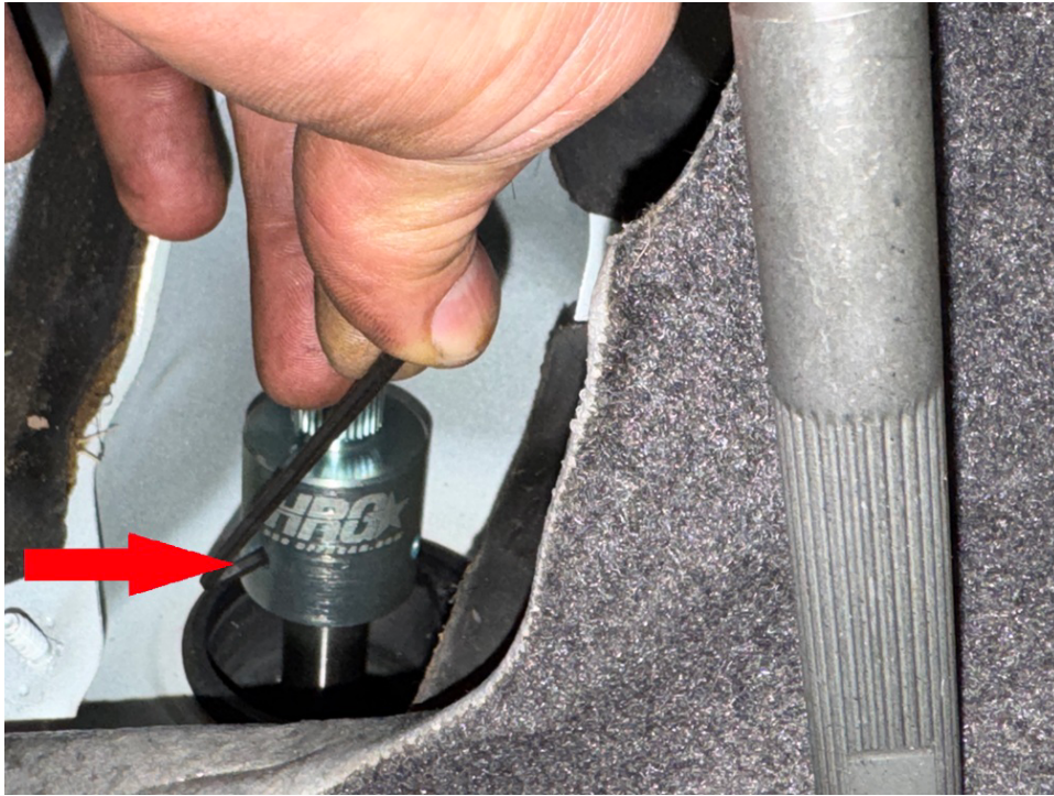
Step 16. Install foam weather seal between steering rack and body.
