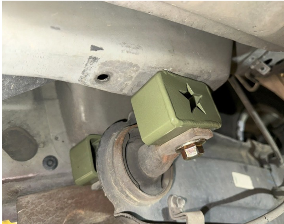
Step 11. Install extended exhaust hangers on both mufflers as shown:
