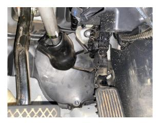
Step 12. Using a body saw, trim sheet metal for clearance around steering coupler. This can also be done by simply bending the sheet metal back about 1/2 inch around the coupler. Turn steering wheel to verify the coupler has proper clearance.
