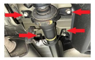
Step 6. Remove one M14 bolt and loosen second M14 bolt in driver side rear trailing arm. Install 1.25x1" M14 spacers one at a time and replace OEM bolts with supplied M14x90 bolts.
