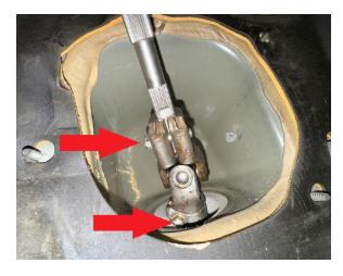
Step 13. Install foam weather seal between steering rack and body.
