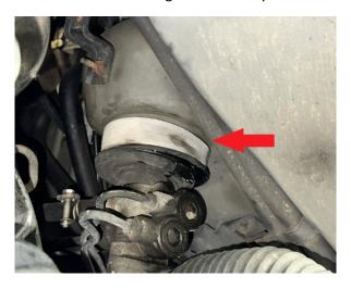
Step 14. Re-install dust cover on steering column below interior dashboard.
