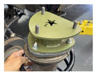
Step 24. Reinstall strut in reverse order, using supplied M10 nuts to attach spacer to body.
