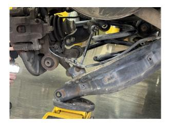
Step 16. Install spacer on the top of the spring, between the spring and the spring seat. Re-use rubber spring isolator. (See diagram below.)
