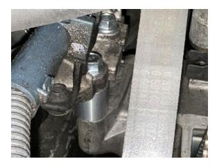
Step 10. Trim plastic splash shield as necessary to fit with lowered subframe, reinstall using original hardware.
