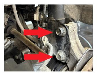
Step 21. Using a length of wire, or large zip ties, temporarily secure hub so as to prevent axle shaft from slipping out of inner hub.
