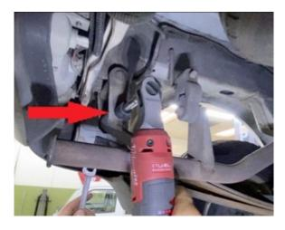
Step 7. Slide 2 M10 bolt sleeves through OEM rubber bushings.
