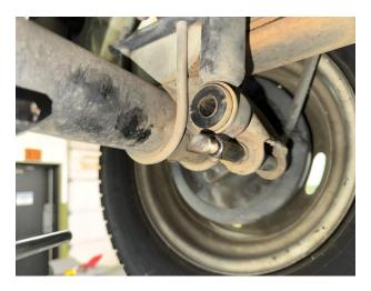
Step 5. Lower rear axle about 2 inches, taking care not to lower more than that to protect rear brake line.
