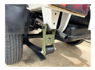
Step 10. Place shock extension onto shock mounting stud. Reuse OEM hardware.
