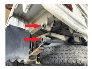
Step 8. Push new extended spring shackle over rubber bushings and align bolt holes.
