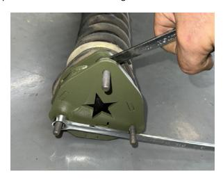
Step 8. Install spacer/strut combo using hardware provided in the kit. Be sure spacer is oriented as shown!
