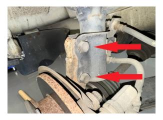
Step 3. Remove 12mm bolt holding brake lines to strut.
