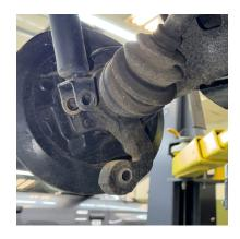
Step 5. Lower jack to release pressure on the spring. Remove spring.
