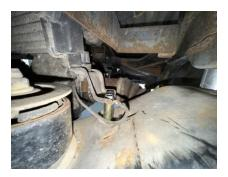
Step 18. Remove 14mm pinch bolt holding passenger (LEFT) side knuckle to strut.
