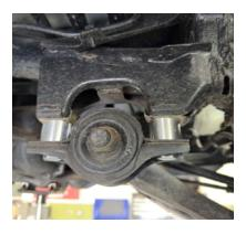
Step 14. Remove bolts holding front differential to crossmember.
