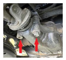
Step 15. Place 2 1x1 M10 spacers between front differential and frame, secure with M10x110 bolts. (see photo)
