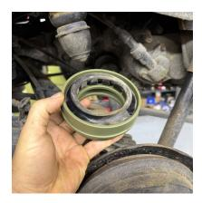
Step 7. Install spring and spacer as shown:
