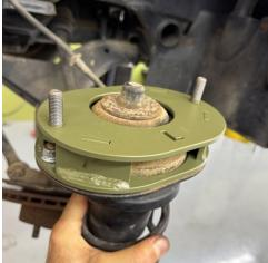
Step 26. Mount spacer/strut assembly into vehicle using original hardware. The top of the strut will spin. Turn the top of the strut so that the L faces OUT. Installing the spacer backward will result in extreme positive camber.
