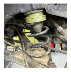
Step 8. Lift suspension arm with jack to compress spring.
