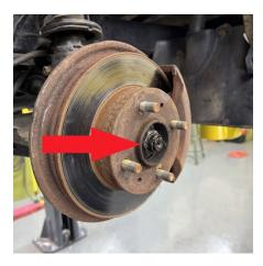
Step 21. Using a heavy hammer, tap on knuckle to slide off of strut.
