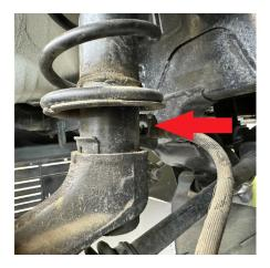
Step 20. Using a 30mm socket, remove axle nut.
