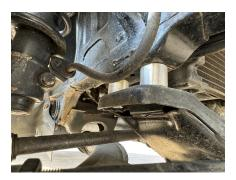
Step 12. Remove bolts holding front lower control arm to frame, and thread in 1 M12x45 bolt on each side.
