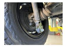
Step 10. With rear suspension compressed, tighten bolt holding rear arm to frame.
