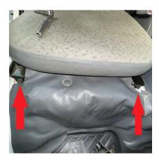
Step 31. Slide seat all the way forward, and remove 2 rear bolts.
