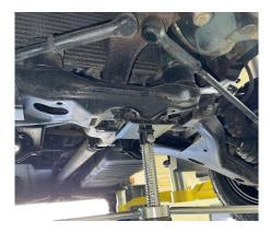
Step 9. Remove bolts holding subframe to body, and temporarily thread M12x45 bolts in their place, 1 on driver side and 1 on passenger side.
