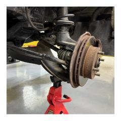
Step 28. Reinstall 14mm pinch bolt and 12mm bolt holding brake line to strut.
