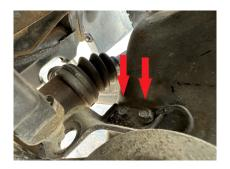
Step 17. Install 05.x1 M6 spacers and M6x40 bolts as shown. Be sure to reconnect ground wire!
