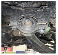
Step 13. Place 1.25x1 M12 spacers between front lower control arm and frame and secure with M12x45 bolts as shown in photo:
