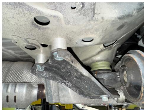
Step 11. Install 8 1.25x1 M12 steel spacers between main subframe bolt retainer brackets and body using supplied M12x50 bolts. (see photo)
