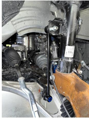
Step 38. Double check all bolts. Especially sway bar links!
