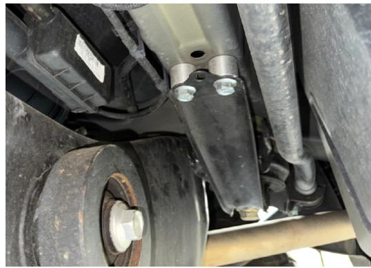
Step 5. Remove rear 2 subframe bolts one by one, installing remaining 3.5x1 spacers and installing M14x160 bolts.
