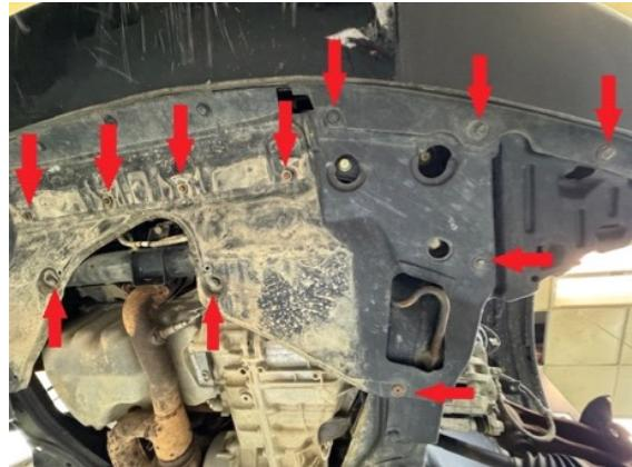
Step 6. Remove plastic clips and 10mm bolts holding aluminum heat shield behind subframe. (IF APPLICABLE) Save hardware.
