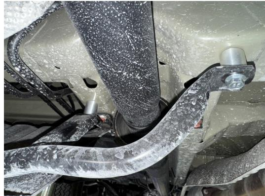
Step 14. Tighten 10mm bolts on plastic under tray.
