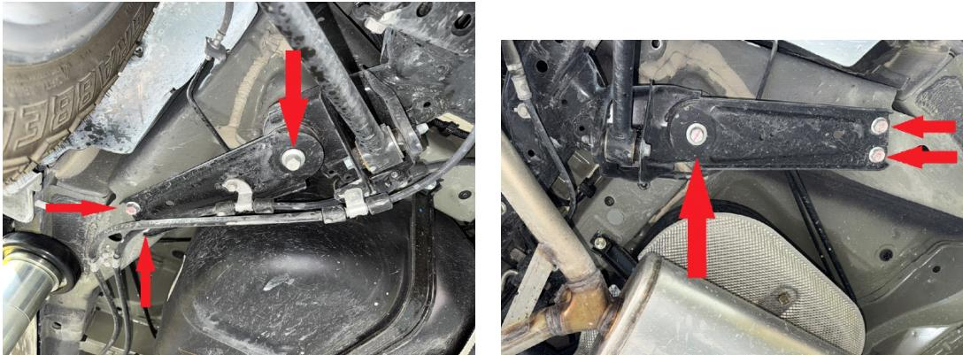
Step 4. Loosen 4 main M14 bolts holding subframe to body, removing only the front 2. This allows the subframe to drop enough to install 2 of the 4 3.5x1" M14 spacers between subframe and body. Install M14x160 bolts. Be sure to pass bolts through support brackets! (see photo)
