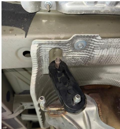
***NOTE: It is not necessary to modify the exhaust hanger that is attached to the rear subframe.***
