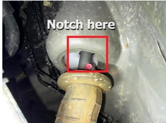
*ALTERNATE METHOD: Using a screwdriver or round bar, bend sheet metal back about 1/4 inch around the coupler. Turn steering wheel to verify the coupler has proper clearance.*
