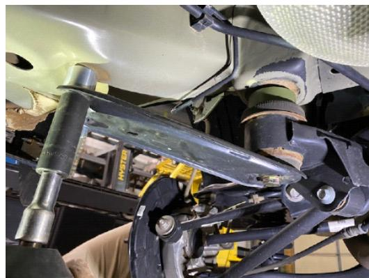
Step 7. Remove driveshaft protector loop.
