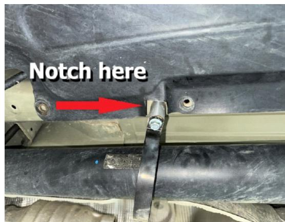
Step 9. Remove 2 14mm bolts holding driveshaft carrier bearing, and 12mm bolt holding gas tank bar.
