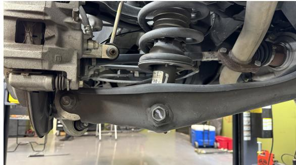
Step 27. Reinstall bolt holding lower control arm to hub. Torque bolts to 135 ft-lb.
