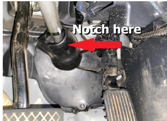
Step 18. Re-install dust cover on steering column below interior dashboard. Double check full rotation of steering wheel to check for any noises or rubbing. Trim as necessary.
