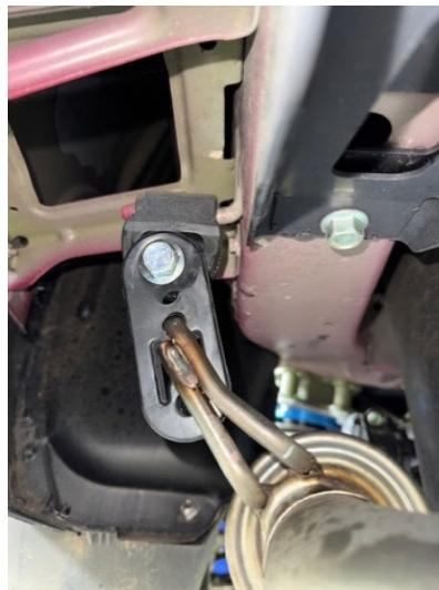
Step 17. Remove rubber hanger from exhaust mid-section under vehicle.
