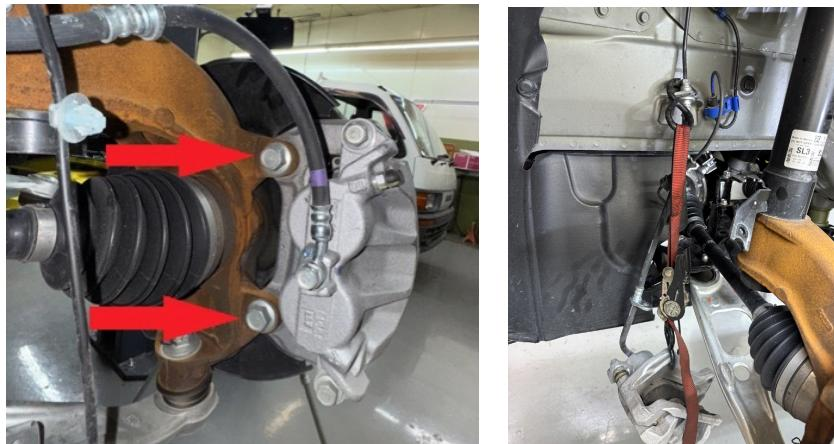
Step 23. Remove brake rotor and axle nut.
