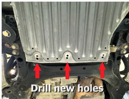
Step 14. Re-install aluminum heat shield, bend as necessary to fit with lowered subframe. Re-attach using OEM hardware.
