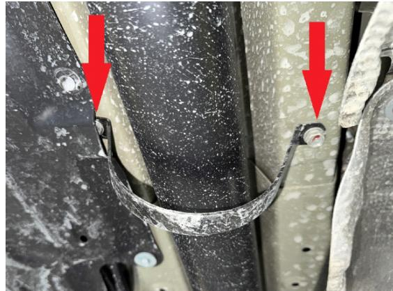
Step 8. Cut notch in plastic and install 0.75x1 M8 spacers and M8x40 bolts as shown.
