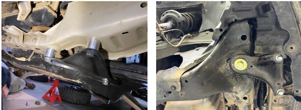
Step 12. Trim plastic splash shield as necessary to fit with lowered subframe, reinstall using original hardware.
