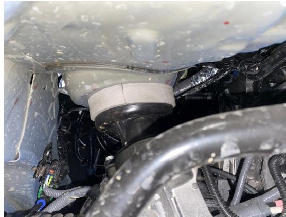
Step 17. Under driver side dash, remove plastic dust cover on steering column to gain access to steering coupler.
