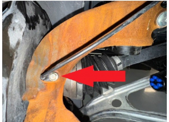
Step 18. Remove nut holding tie rod end to hub, strike knuckle with heavy hammer to dislodge tie rod end.
