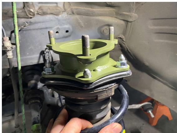
Step 33. Spin strut top 180\* and slide studs on spacer through original mounting holes in strut tower. Secure strut spacer with OEM hardware. Tighten nuts to 33 ft-lb.
