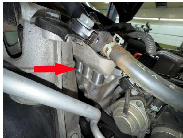
Step 17. Reinstall engine bracket using M14x100 bolts. (see diagram)
