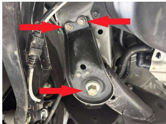
Step 7. Remove driver side rear main subframe bolt. Temporarily thread in a M14x160 bolt included in the kit. (see photos)
