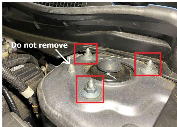
Step 32. Place strut spacer on top of strut and secure with hardware provided in the kit.
