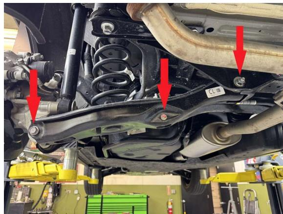
Step 17. Remove spring and place lift spacer on top of rubber isolator as shown.
