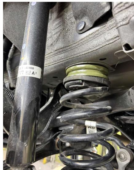
Step 19. Place rear shock spacer between rear shock and body, install M8x60 bolts. torque bolts to 30 ft-lb
