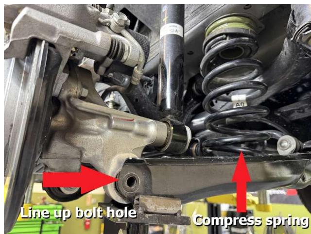
Step 21. Reinstall bolt holding lower control arm to wheel hub.
