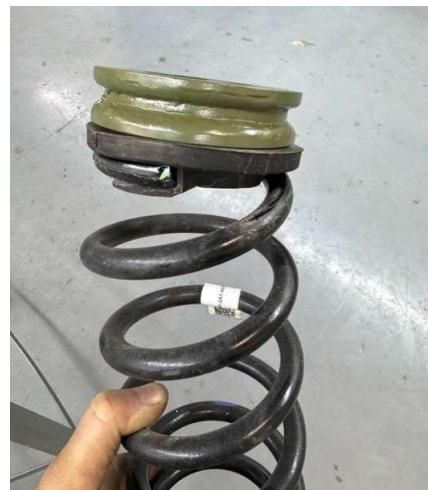
Step 18. Reinstall spring and spacer. Be sure lower spring coil is rotated properly and fully seated in the lower rubber isolator.
