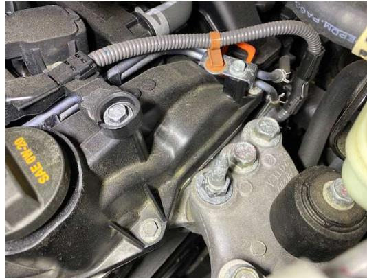
Step 9. Remove subframe bolts shown in photos below (both driver and passenger side)
