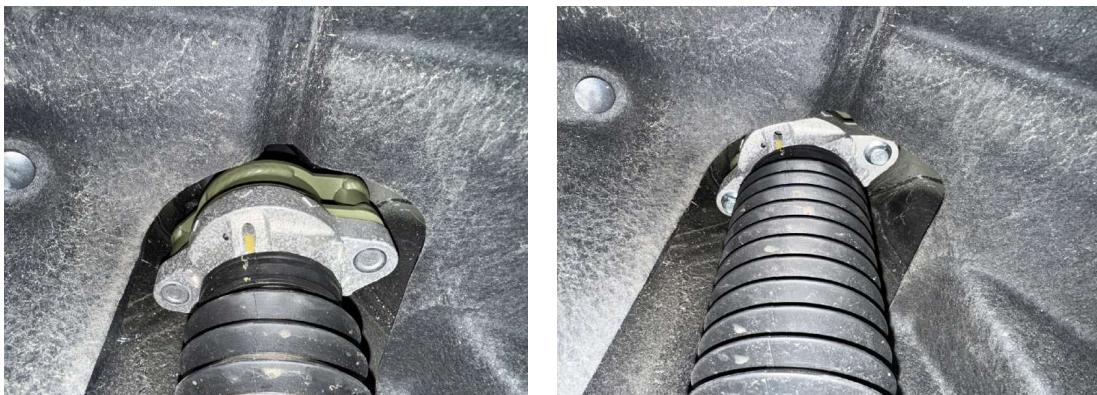
Step 20. Use jack to compress the spring and raise the lower control arm back into place.
