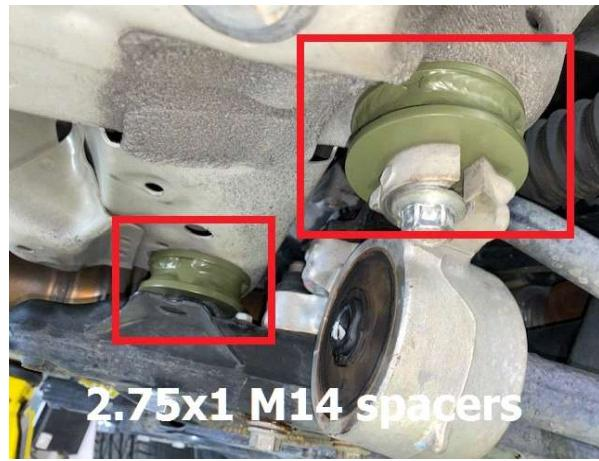
Step 12. Install M14x115 bolts in place of OEM bolts to secure subframe in place
