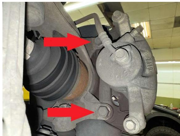
Step 26. Remove brake lines and ABS wiring, remove wheel sensor from knuckle.
