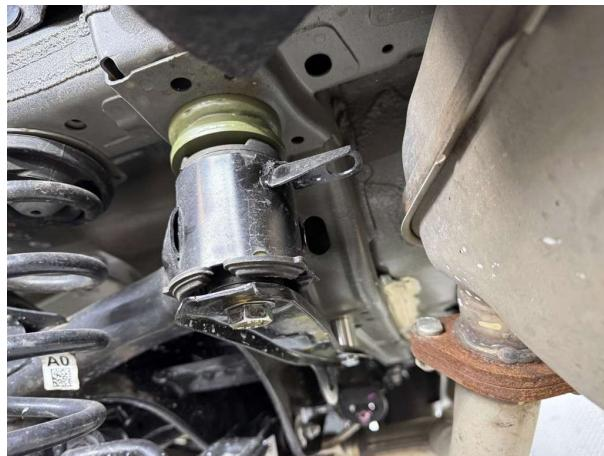
Step 12. Remove 2 bolts holding driver side trailing arm to body.
