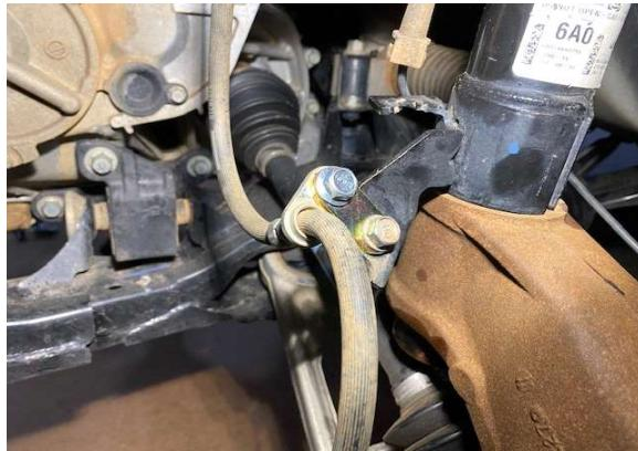
Step 40. Reinstall ABS wire, wheel sensor, and brake line. Tighten brake line mounting bolts to 25 ft-lb.
