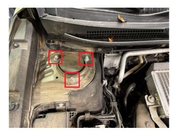
Step 7. Mount driver side (L) spacer to strut using M8 nuts provided in the kit.
