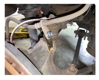
Step 19. Replace OEM muffler hangers with extended ones provided in the kit.
