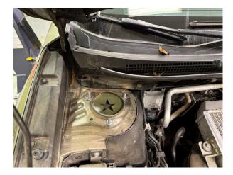
Step 10. Mount ABS and brake lines back to strut, use BLBL (L shape bracket) to relocate front brake line.
