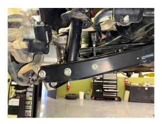
Step 18. Install rear brake line extension bracket in factory brake line mounting location. Mount brake line as shown:
