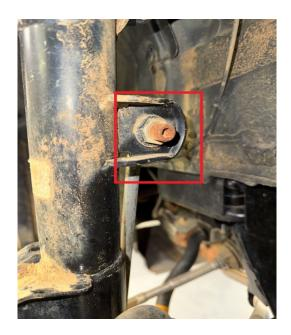
Step 6. Remove 3 M8 nuts from strut top to allow strut to drop out. (save hardware).
