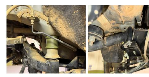
Step 11. Remove bolts holding sway bar link, rear strut, and wheel hub to driver side lower control arm. (see photo)
