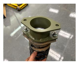
Step 15. Slide strut back into vehicle and install the strut assembly using the hardware provided.
