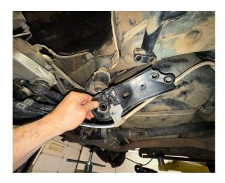
Step 6. Remove front-most main subframe bolts, temporarily replace OEM bolts with M14x220 bolts provided in the kit. These will keep the subframe in line while being lowered.
