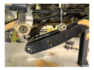
Step 12. Remove brake line from hub to prevent tension on the hose while lowering wheel hub.
