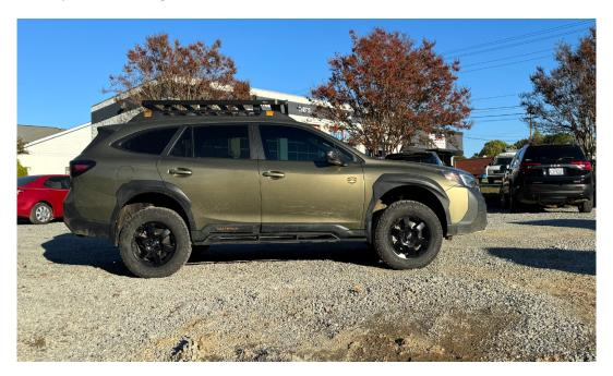
Note: Installing lift spacers will change the suspension geometry and will require a 4 wheel alignment.
