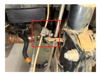
Step 5. Remove sway bar link from strut. (save hardware) You will not reconnect the sway bar link until both sides are lifted.
