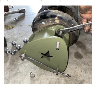
NOTE: The spacers in this kit are offset to maintain proper camber/caster alignment, and are marked L for driver side and R for passenger side.
