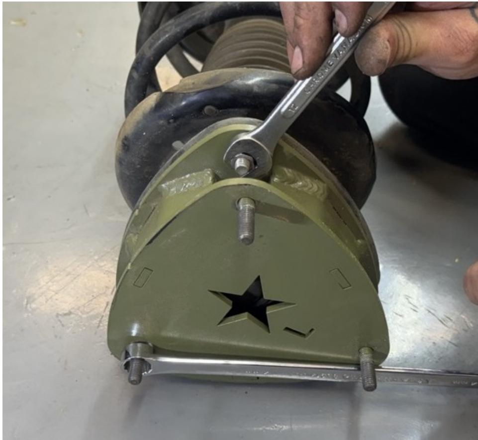
Step 8. Slide driver side strut back into place and mount to vehicle using hardware provided in the kit. Torque bolts to 35 ft-lb. **Be sure L is facing as shown in the photo.**
