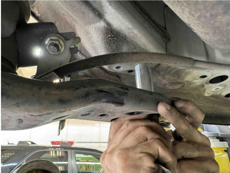
Step 10. Reinstall plastic gas tank covers. Some of the original bolts will not be reused. The support bars will install on the outside of the covers as shown in photo.
