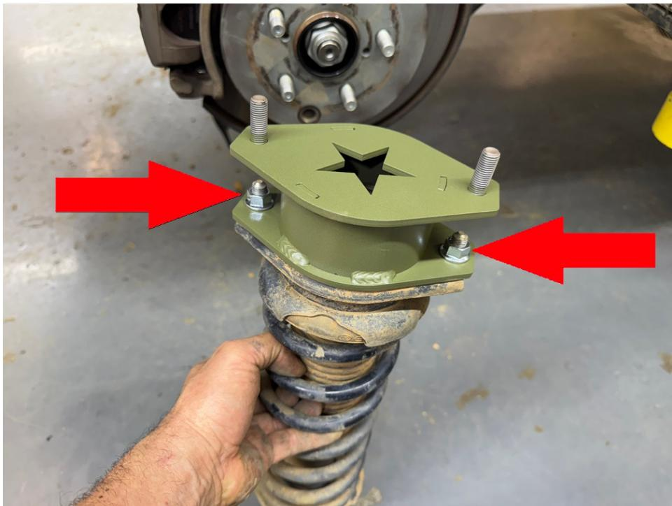
Step 20. Slide strut back into vehicle and install the strut assembly using the nuts saved from step 2.
