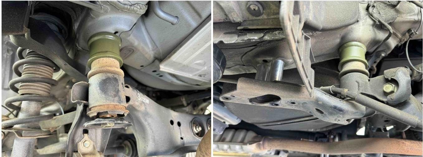
Step 9. Place 2 1x2 M10 spacers between subframe bracket and body, install 2 M10x70 bolts. Torque to 50 Ft-Lb.
