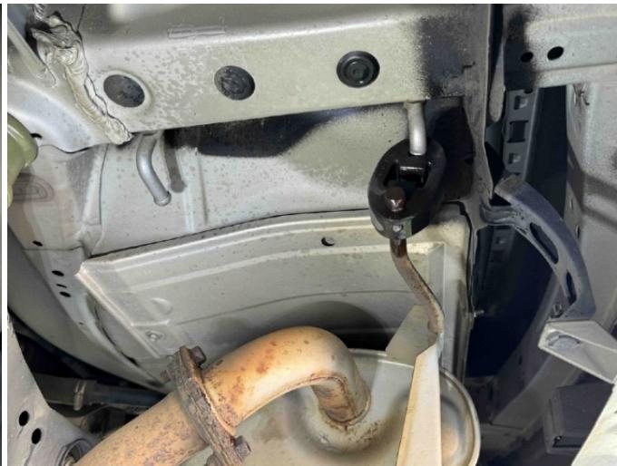
Step 25. Install new muffler hangers as shown in photo:
