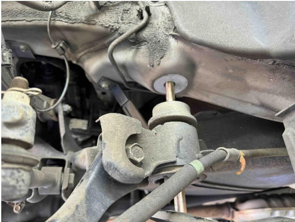
Step 7. Place 2.75x2 M14 spacer between subframe and body, install M14x200 bolt, repeat process for both sides. Torque bolts to 85+ Ft-lb.
