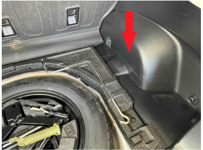
Step 13. Pull up cargo liner and remove plastic panels to gain access to rear strut bolts.
