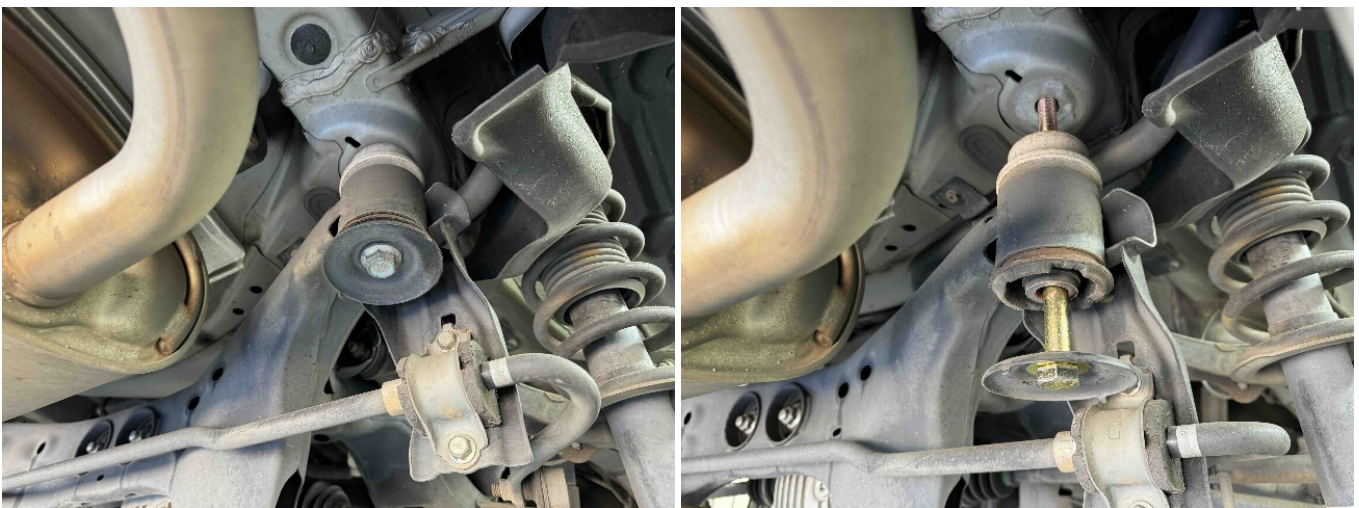
Step 5. Locate and remove 2 of the 4 main rear subframe bolts. Replace with 2 new bolts provided in the kit to keep the subframe square and in line while lowering.
