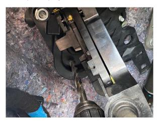
Step 14. Using pliers, unplug wiring from switch as shown. DO NOT PULL ON WIRING.
