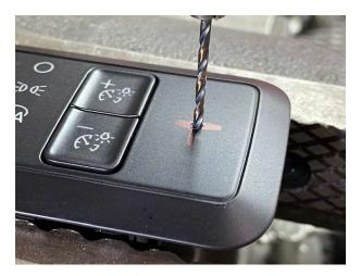
Step 23. Using a large unibit, drill hole out to 7/8" (Be careful not to go over)
