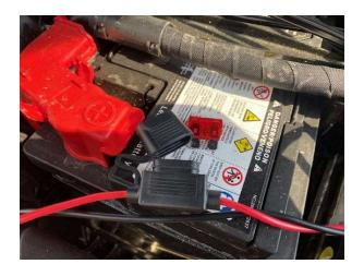
Step 10. Connect main power cable to positive battery stud.
