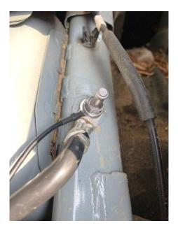
Step 12. Remove parking brake override housing from firewall.
