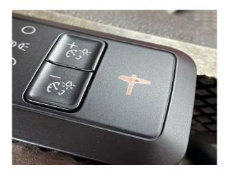
Step 22. Using a 1/8" bit, drill pilot hole.
