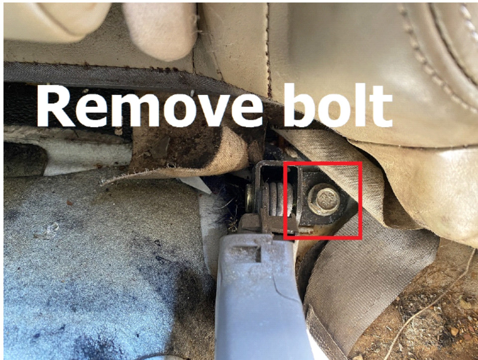
Step 3. Remove 4 12mm bolts holding seat back to floor.
