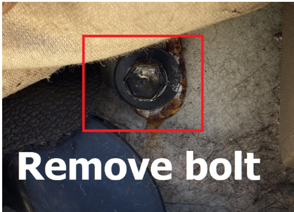
Step 4. Lift up rear seat back to remove, exposing rear strut mounting bolts. These will be removed in step 9.
