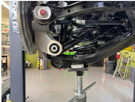
Step 11. Place lift spacer on top of spring.
