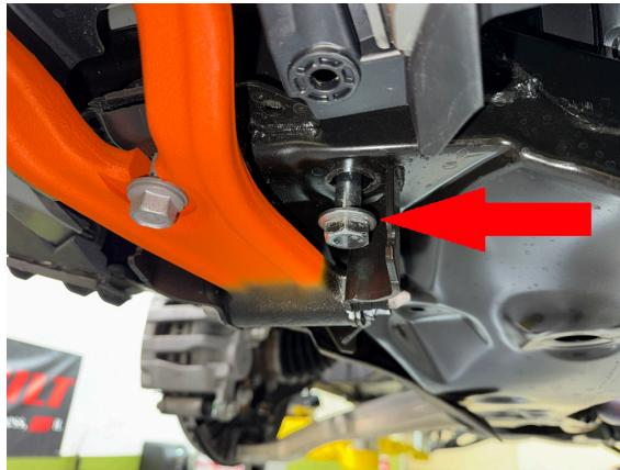
Step 9. Remove the "rear-most" 2 front subframe bolts and temporarily replace them with 2 of the new M14x150 bolts that come with the kit.
