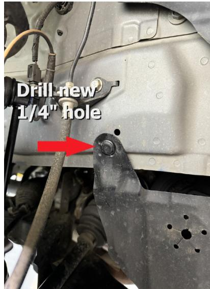
Step 16. Drill as needed to enlarge holes in plastic to help align clips.
