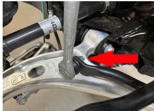
Step 7. Remove lower ball joint nut and cotter pin.
