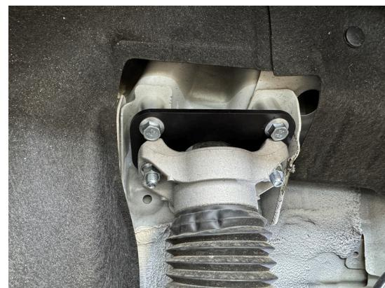
Step 17. Bend ABS wire mounting bracket as shown.
