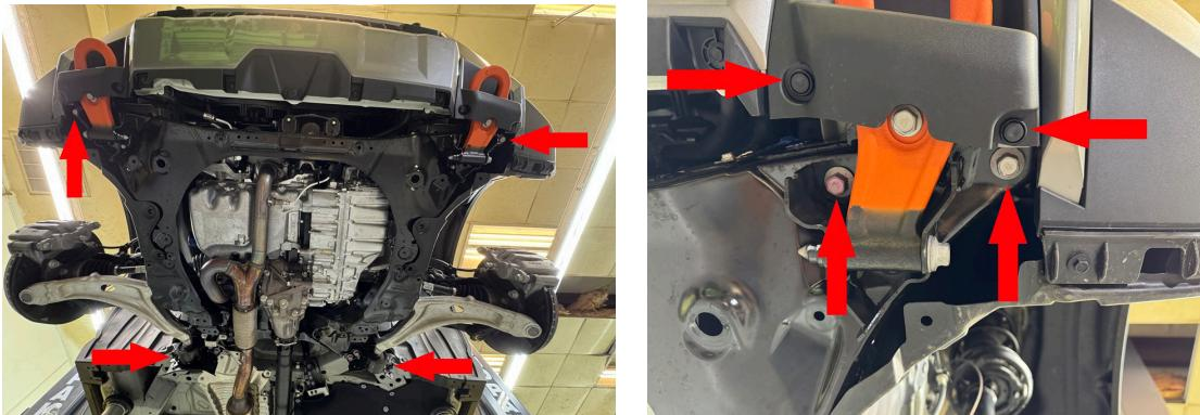
Step 8. Remove 2 of the "front most" 4 main subframe bolts and temporarily replace them with 1 M14x160 bolt on the driver side and 1 M14x160 bolt on the passenger side to keep the subframe in line when being lowered.
