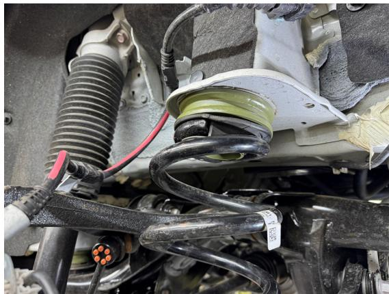
Step 12. Using a floor jack, compress spring until bolt holes line up, reinstall bolt.
