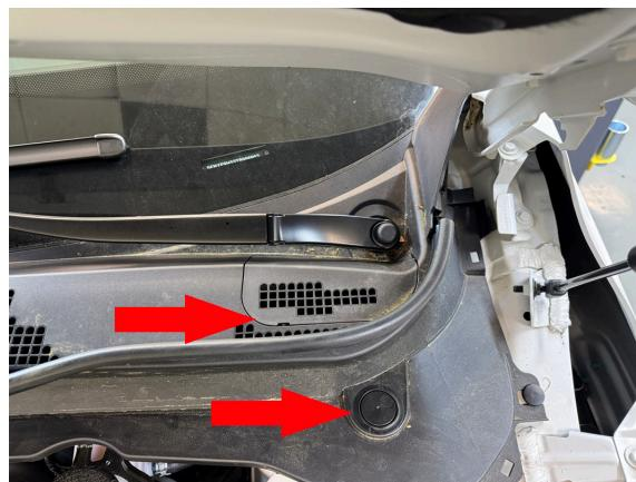
Step 10. Remove 14mm nuts holding struts to body, remove strut and hub assembly as one piece. **Do not separate strut from hub.**
