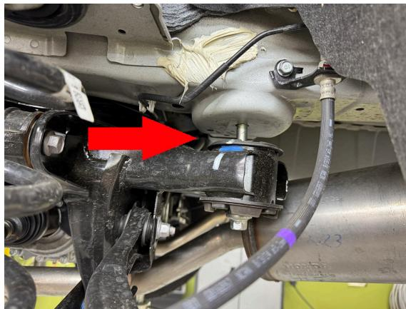
Step 10. Using the floor jack, carefully lower subframe approximately  $\frac{1}{2}$  inch.
