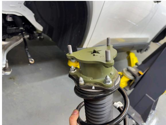
Step 29. Mount spacer, strut, and hub assembly back into shock tower using M10 nuts provided in the kit as shown. Torque nuts to 33 ft-lb. BE SURE THE SPACERS ARE CLOCKED AS SHOWN. THESE SPACERS HAVE BUILT IN CAMBER AND CASTER CORRECTION!
