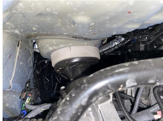
Step 20. Double check all bolts. Torque all main subframe bolts to 135 ft. lb.
