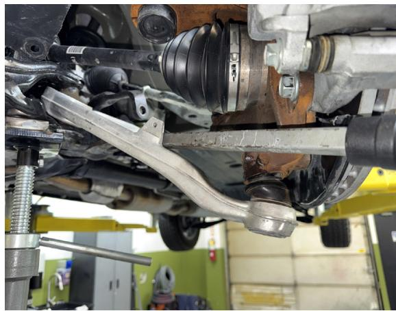
Step 31. Reinstall the lower ball joint nut and cotter pin. Torque to 42 ft-lb and be sure to line up the castle nut with the hole for the cotter pin.
