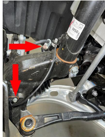
Step 3. Remove nut holding tie rod end to hub, strike knuckle with heavy hammer to dislodge tie rod end.
