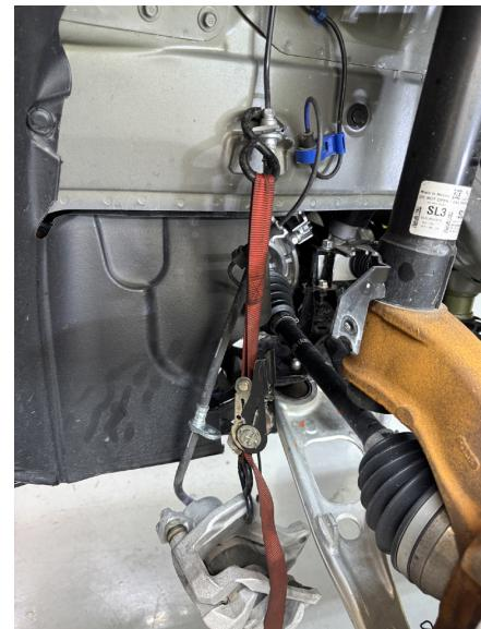
Step 5. Remove brake rotor and axle nut.
