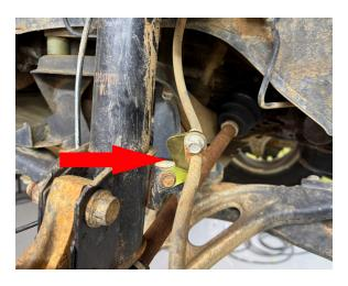
Step 12. Reinstall ABS wiring. Relocate mounting bolt as shown:
