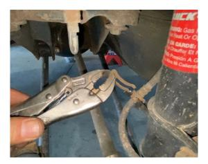
Step 12. Remove 2 19mm bolts at bottom of strut. Save 1 bolt for reinstallation.
