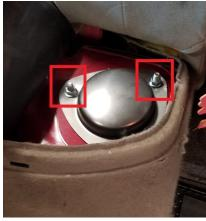
Step 8. Mount the spacer to the strut using the M8 nuts provided in the kit. (See diagram)
