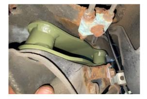
Step 9. Using a floor jack, lift the rear suspension so that the bolt holes for the trailing arm line up with the body, install 3 M12x90 bolts.
