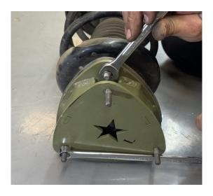
Step 9. Lift strut back into place with the "L" (driver side) facing toward the front bumper and loosely install the original 12mm nuts saved from disassembly. (see photo)
