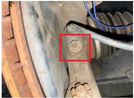
Step 5. Remove brake line from strut. (see photo below)
