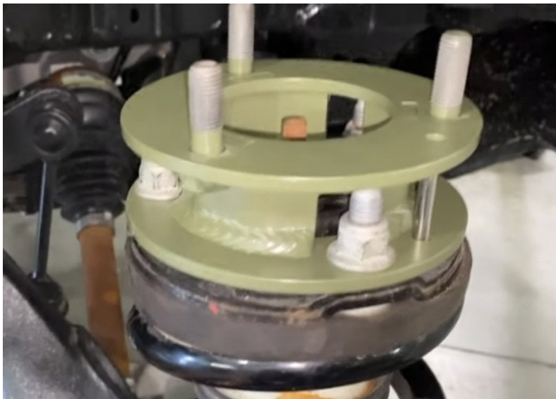
Step 16. Mount strut back into vehicle using hardware provided with the kit.
