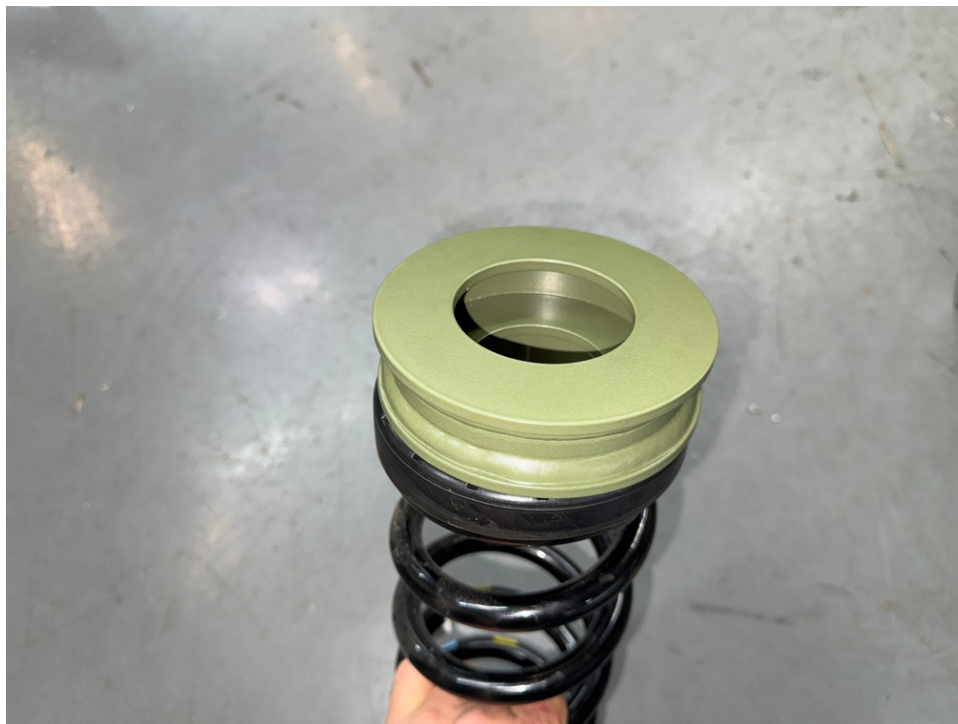
Step 19. Install spring and spacer.
