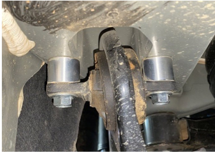
Step 18. Place rubber isolator over rear spring spacer.
