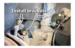
Step 11. Install sway bar link relocation brackets using hardware provided in kit.
