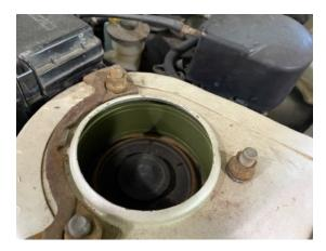
Step 9. Install eccentric bolt (camber adjustment bolt) in place of upper strut mounting bolt, install OEM lower bolt.
