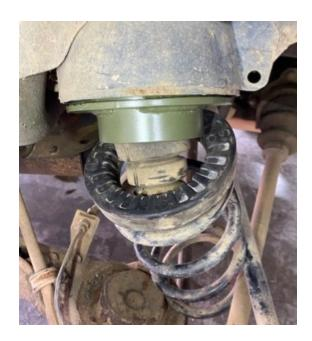
Step 8. Use floor jack to compress the spring and raise the wheel hub back into place.
