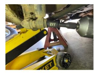
Step 5. Release pressure on spring by lowering wheel hub with floor jack.
