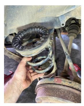
Step 7. Place lift spacer between frame rail and isolator, reinstall spring.
