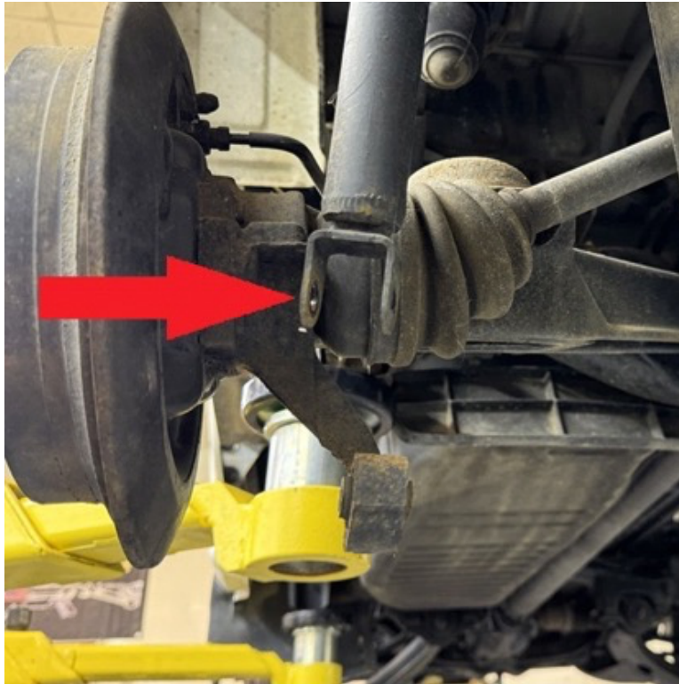
Step 3. Loosen bolt holding rear arm to frame.
