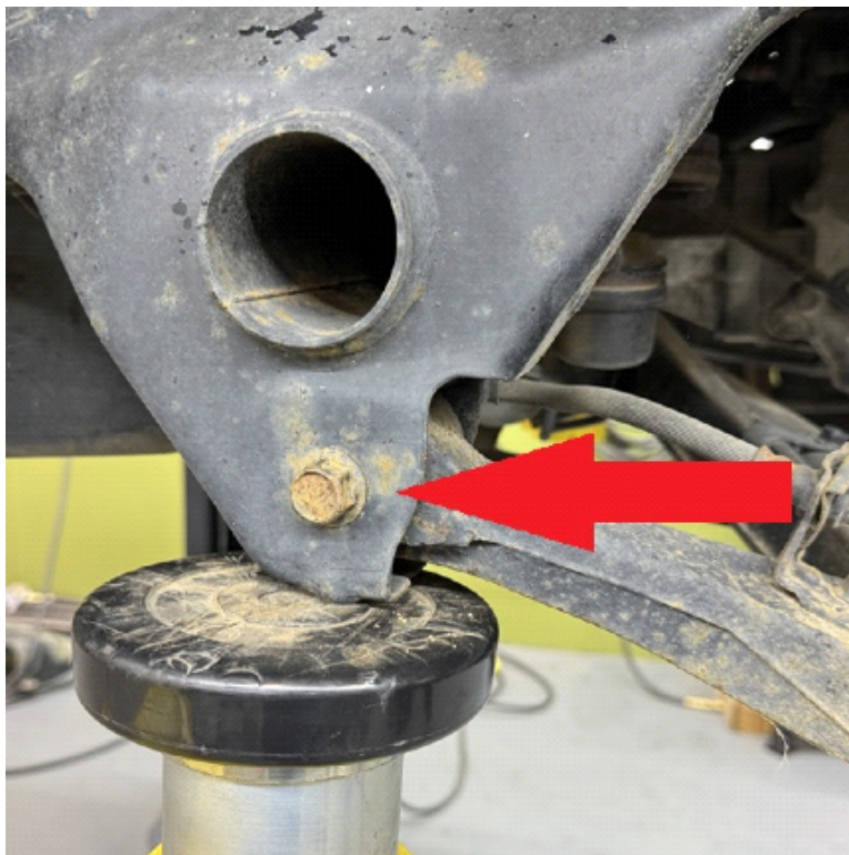
Step 4. Remove bolt holding shock absorber to wheel hub.
