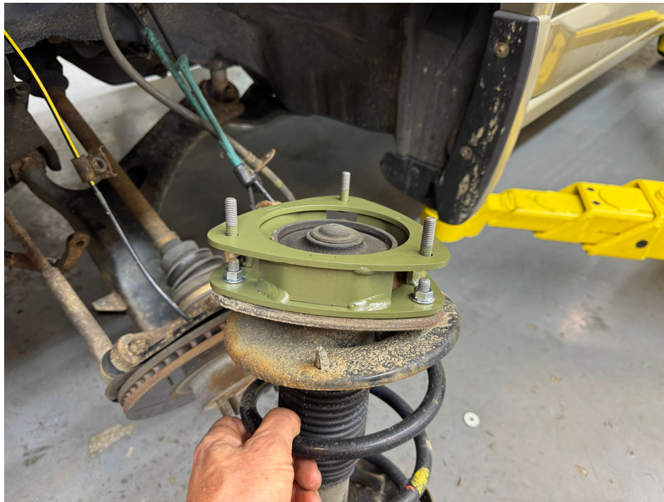
Step 11. Lift strut back into place and bolt in using original hardware. Torque nuts to 25 ft-lb.
