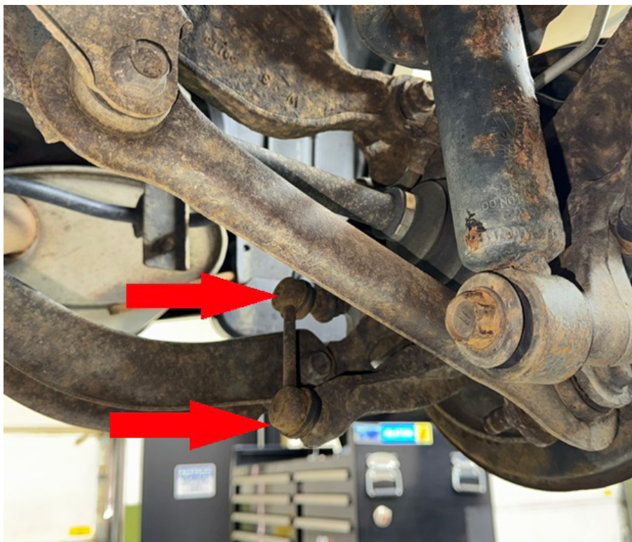
Step 14. Remove bolt holding driver side rear strut to lower control arm.
