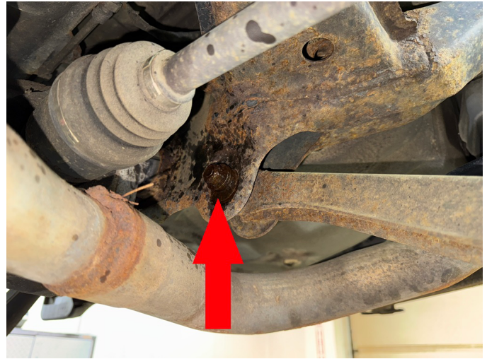
Step 13. Remove both driver and passenger rear sway bar end links. These will not be reused.
