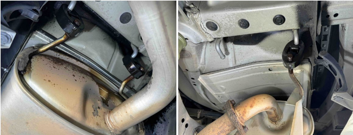
Step 25. Install new muffler hangers as shown in photo:
