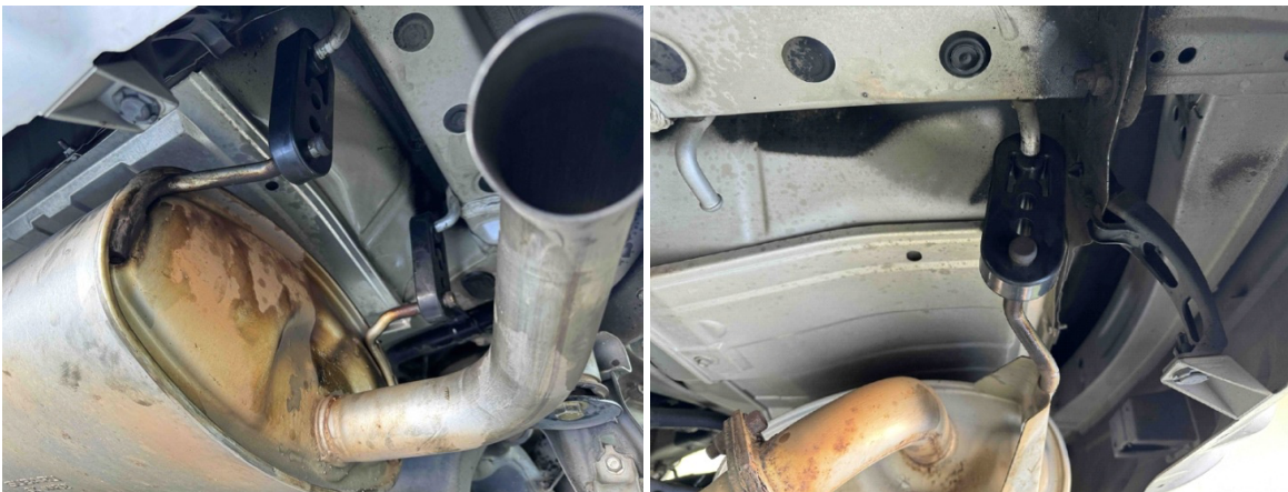
Step 25. Install new muffler hangers as shown in photo:
