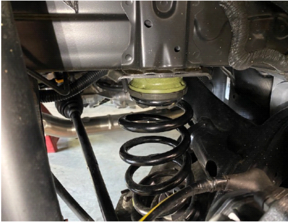
Step 10. Tighten bolts holding swingarms to body
