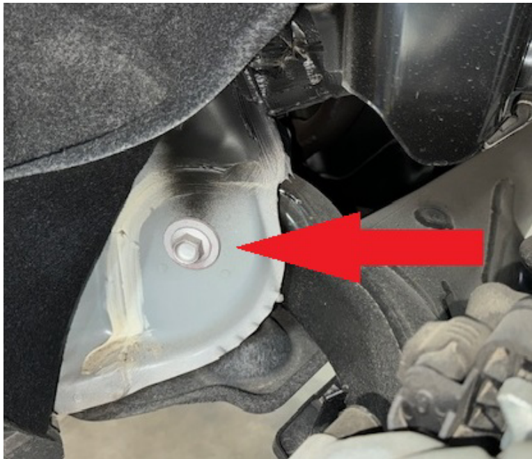
Step 11. Remove nuts holding shock absorber to body.
