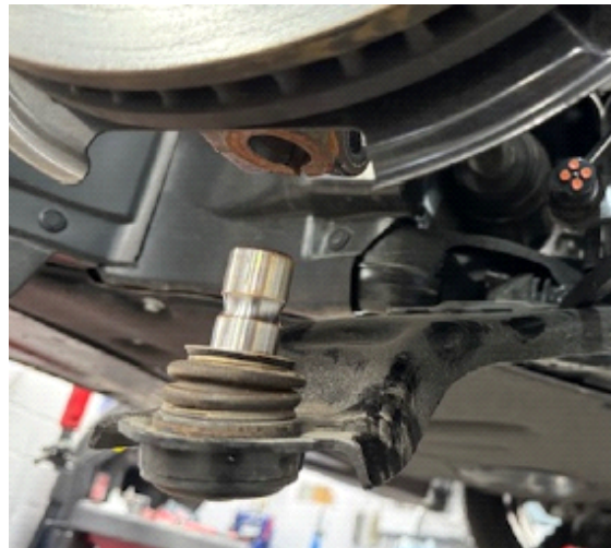
Step 7. Remove cotter pin and loosen nut from tie rod end. Strike knuckle with large hammer to release tie rod end. Remove nut.
