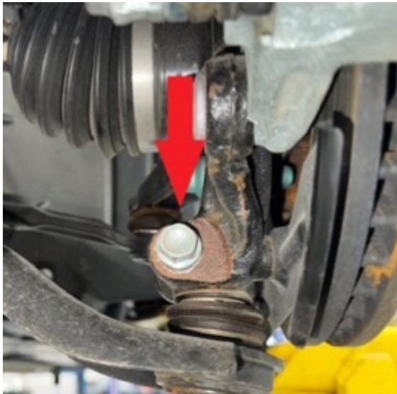
Step 7. Remove cotter pin and loosen nut from tie rod end. Strike knuckle with large hammer to release tie rod end. Remove nut.
