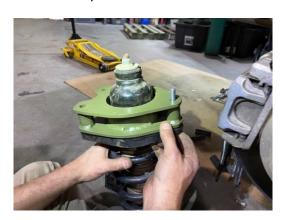
Step 8. Install strut/spacer combination using supplied hardware.
