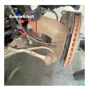
Step 11. Remove lower ball joint nut and using a heavy hammer, strike lower arm to carefully unseat lower ball joint from bottom of hub.
