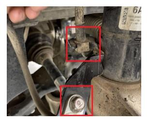
Step 6. Remove nut holding tie rod end to hub, strike knuckle with heavy hammer to dislodge tie rod end.
